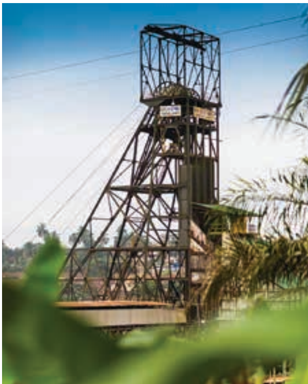
Headgear at the Prestea mine. The mine has been in existence for over 100 years and has historically produced an estimated 9 million ounces of gold (photo: Golden Star Resources).
