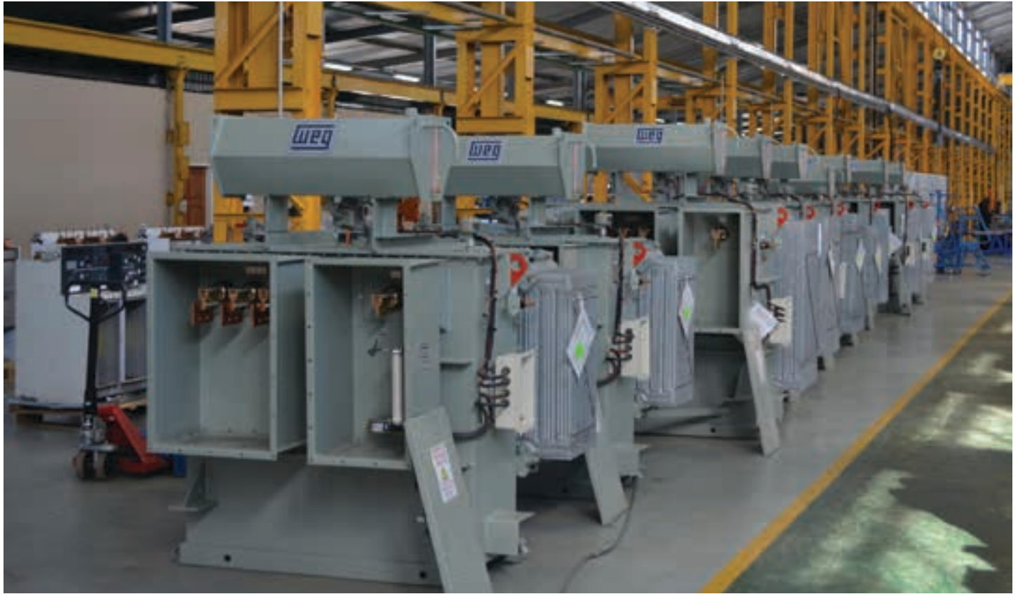
5 x 1 600 kVA 11 kV/433 V and 1 x 2 000 kVA 11 kV/720 V Transformers Export to Ghana
