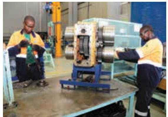
Two technicians assembling a DANA 6000 series transmission used in a Sandvik TH320 dump truck for a customer.
