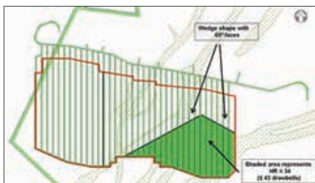
Lift 2 undercut level plan.
