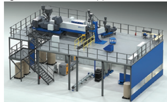
▲ A pilot-scale vertical extrusion group for medium and high voltage cable production in Mailefer's R&D center in Finland
