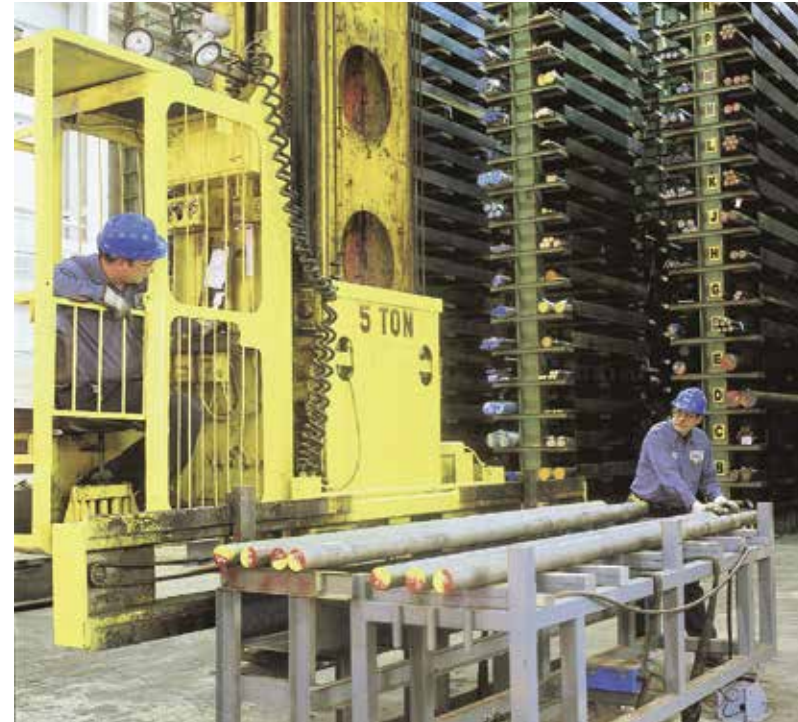
At Service Steel Aerospace, elaborate color coding identifies specialty metals and alloys in the inventory.
