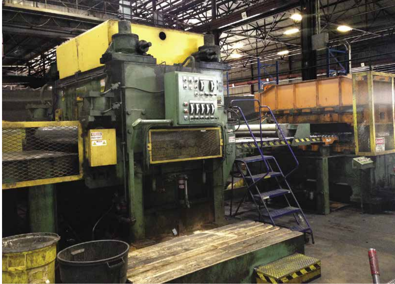
This Herr-Voss cut-to-length leveling line installed at the Los Angeles division was one of the capital investments Reliance made during the 1980s.
