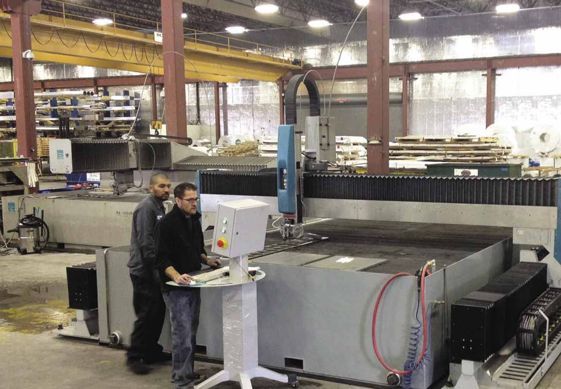
Waterjet cutting at Affiliated Metals, Reliance's last acquisition before the 1994 IPO. This technology uses a high-pressure stream of water mixed with an abrasive to cut metal parts that might be damaged by heat.
