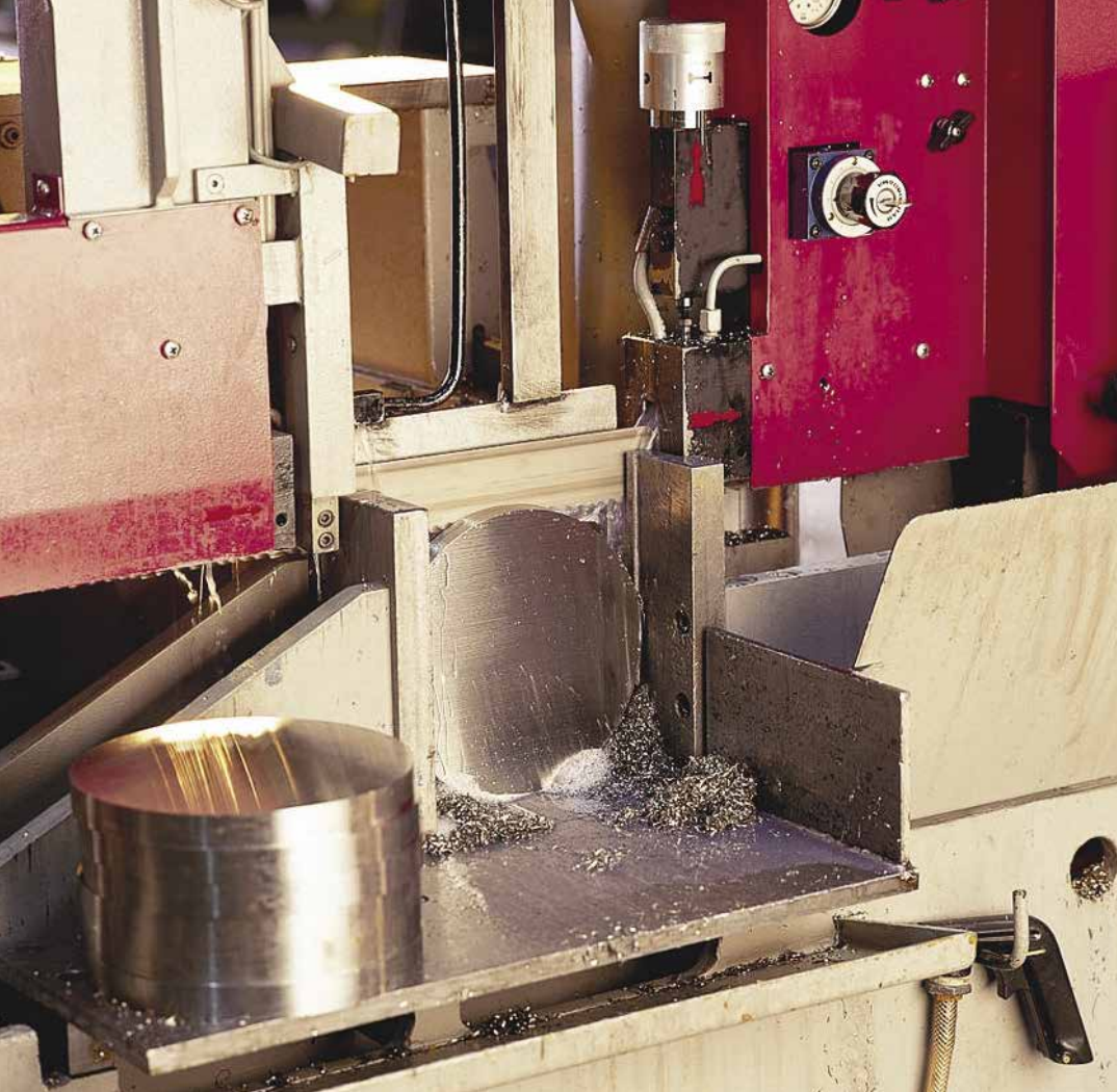
Sawing stainless steel rounds at Service Steel Aerospace, purchased by Reliance in October 1997.
