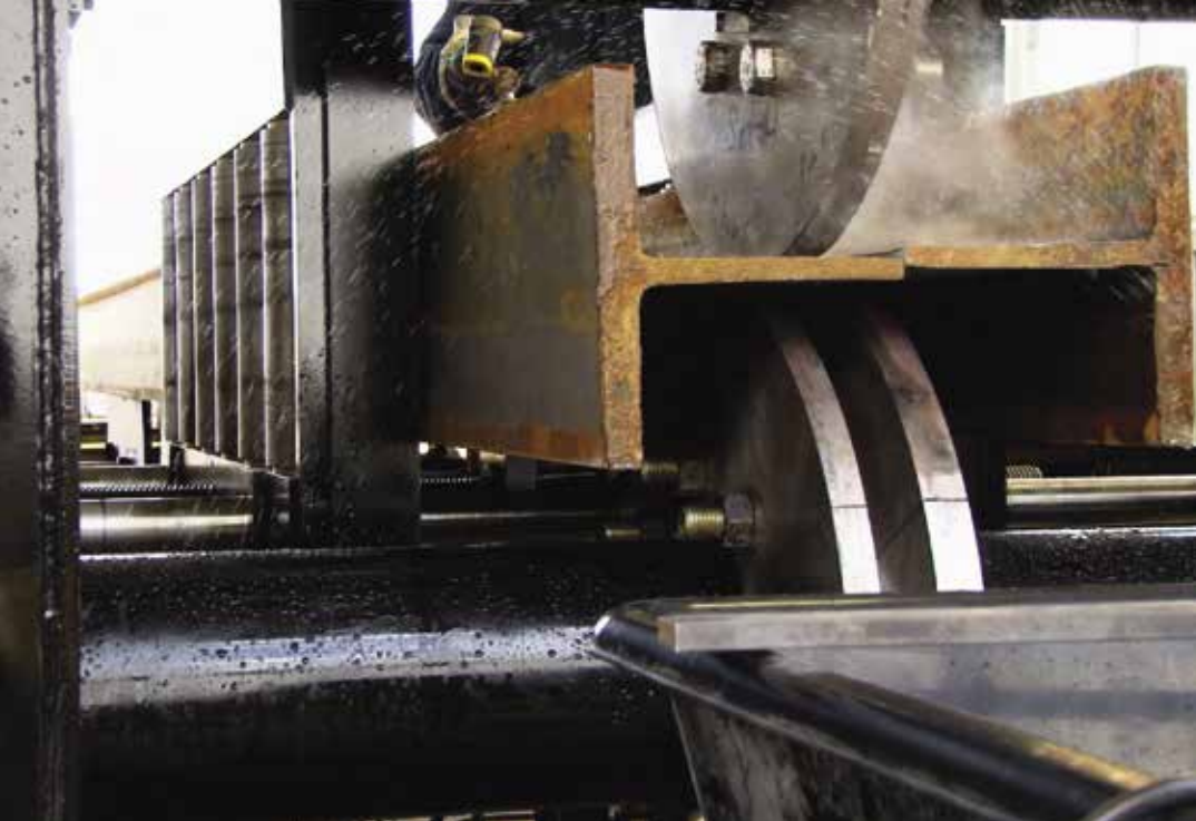
Splitting a steel beam into “tees” using a rotary mechanical shear at PDM, before and after images. A water jet cools the heated steel and keeps particulates down.
