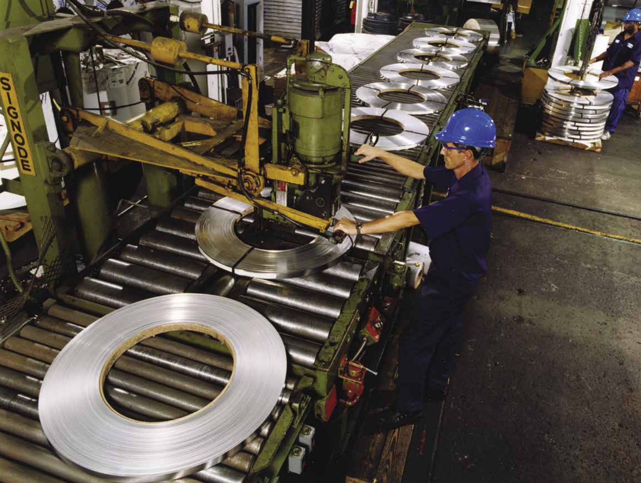
Packaging slit coil on the semi-automatic line at Phoenix Metals.
