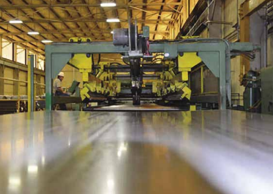
A cut-to-length line at Central Plains Steel, acquired by Reliance in 2002.
