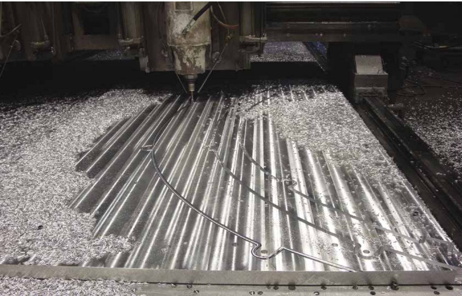
At AMI Metals, a metal plate bound for the aerospace industry goes through the router.
