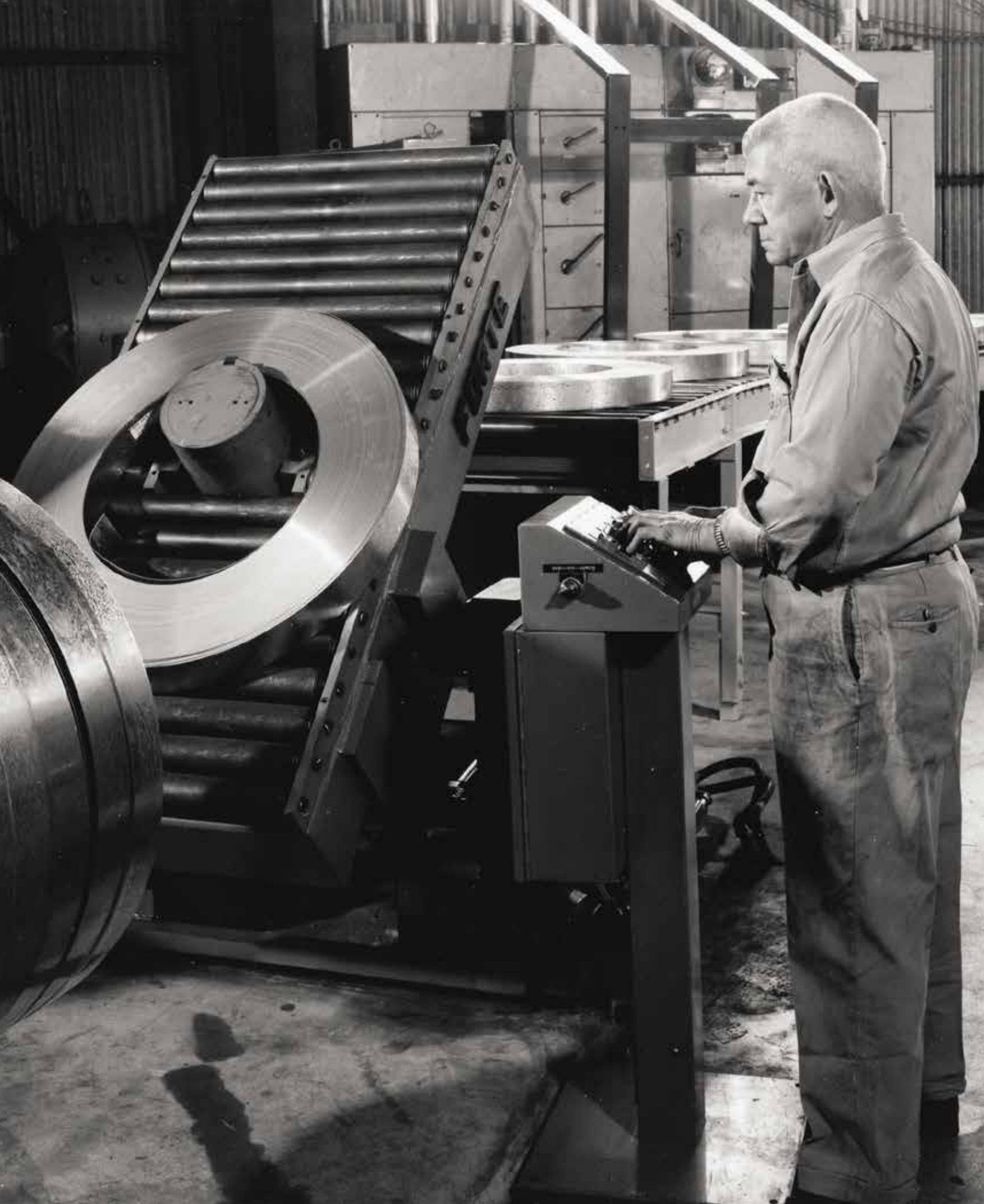
In the Los Angeles metals service center in 1972, an operator uses push buttons to transfer freshly-slit coil from a vertical position to a horizontal position for packaging further down the line.
