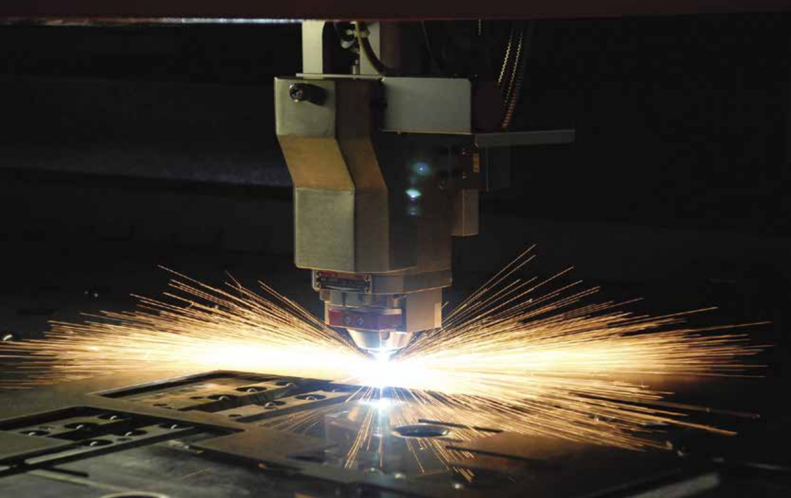
An Amada Pulsar laser cutter at work at Siskin Steel & Supply Company, purchased in October 1996.
