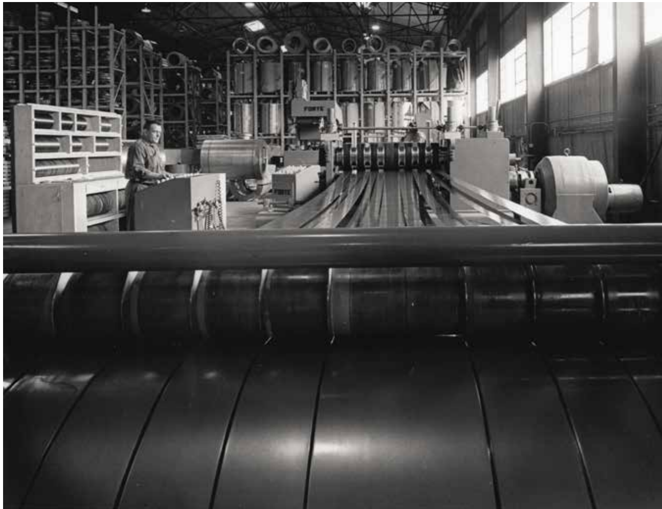
This Cincinnati-Forte slitter installed in the mid-1960s was one of the largest slitters available, capable of processing 20,000-pound coils up to forty-eight inches wide.
