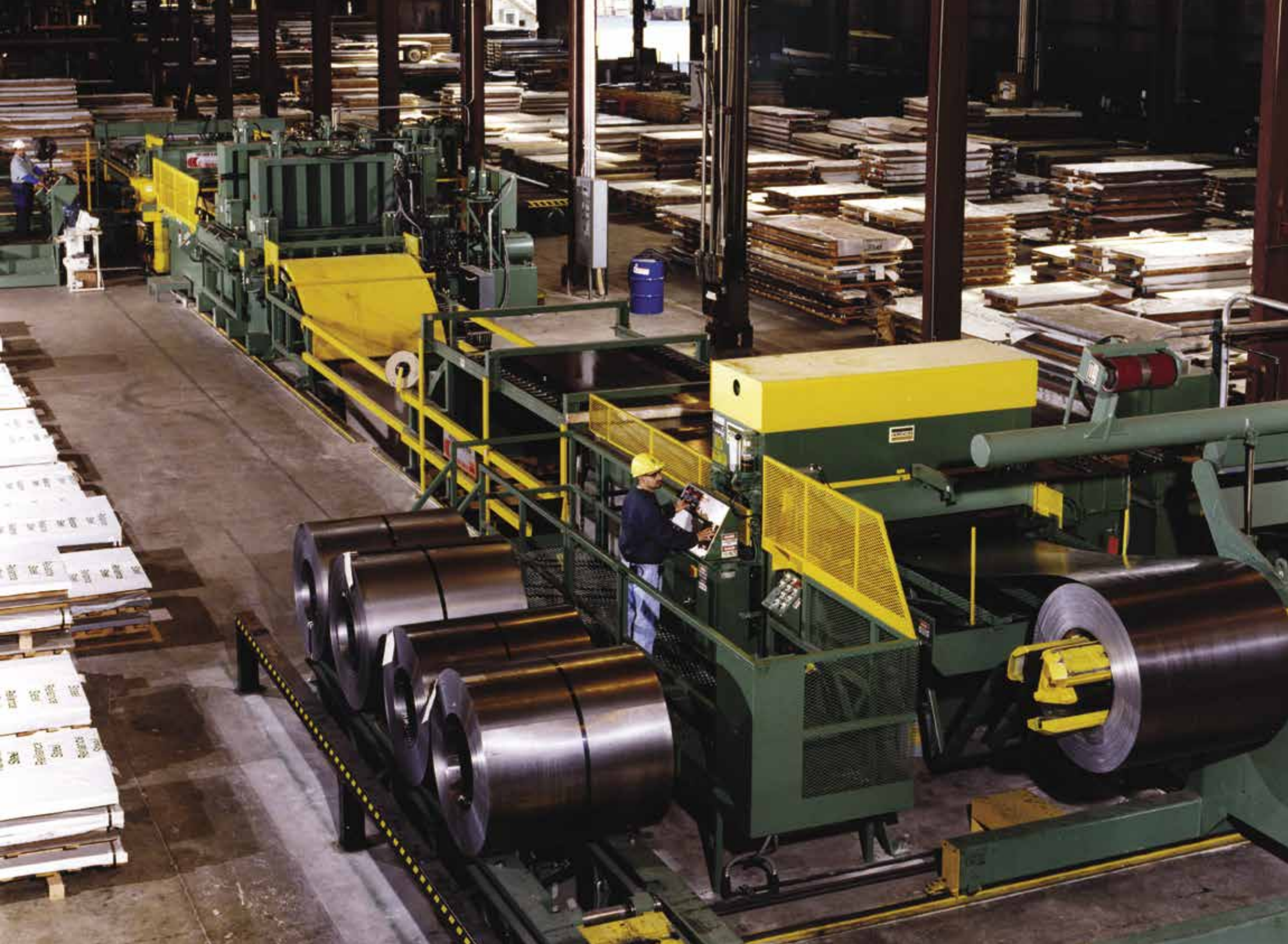
This seventy-two-inch Redbud high-speed multi-cut blanking line was the only one west of the Mississippi River when it was installed at the Los Angeles metals service center in 1999.
