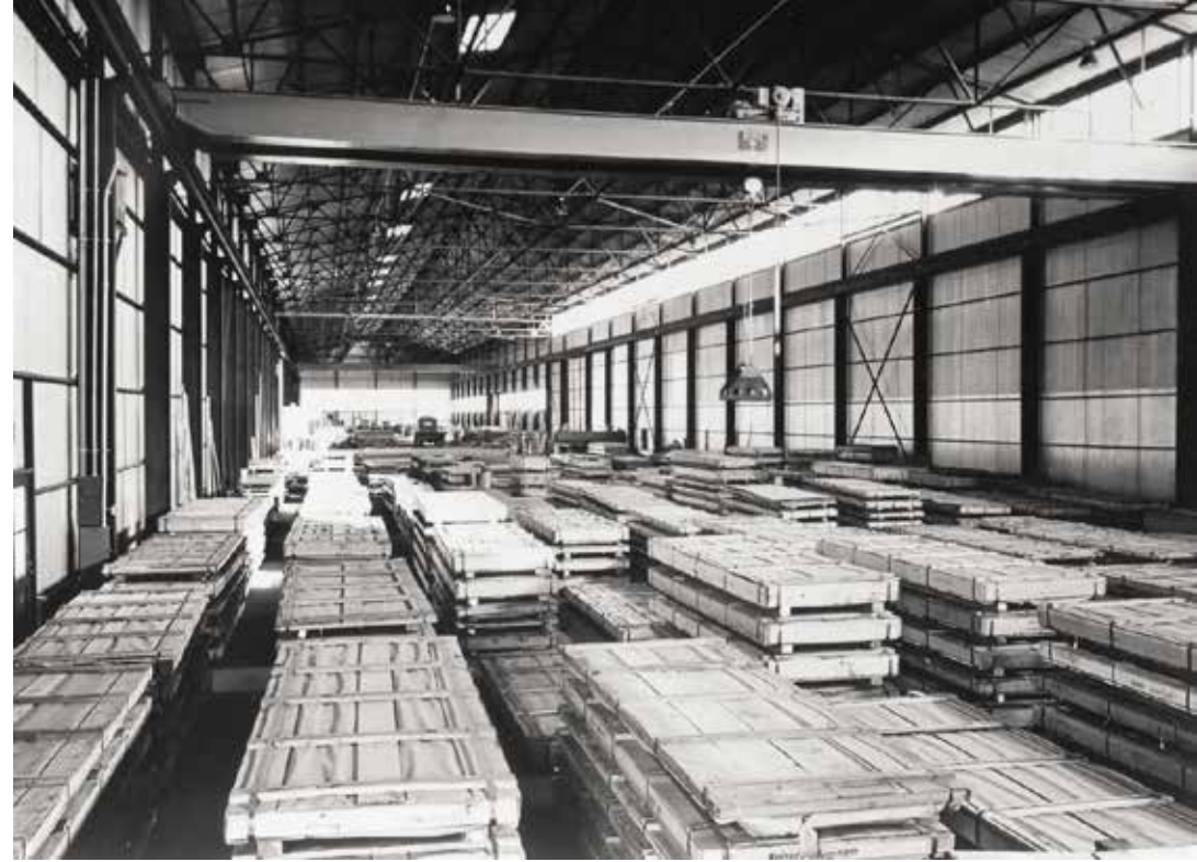
A good example of "unused cube space" during the early 1960s. Stacks of aluminum sheet cover the floor at the Vernon flagship plant while an overhead crane swings in the empty air space above.
