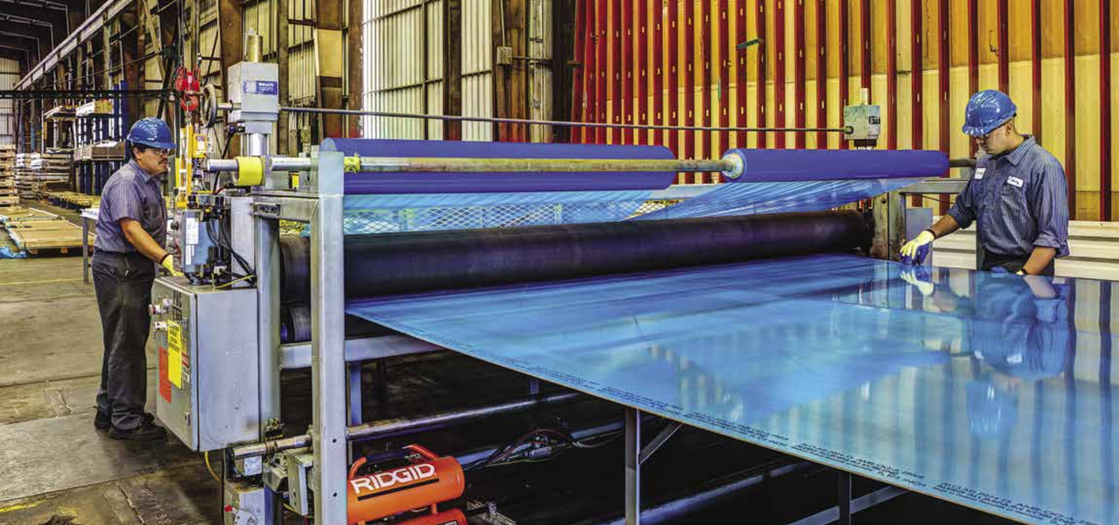
Wide sheet aluminum being covered by polyvinylchloride film at aerospace industry specialist AMI Metals, acquired by Reliance in 1997.
