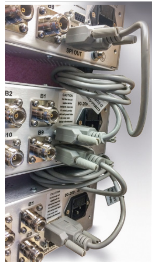
Figure 5: Three units daisy chained via SPI interfaces on rear panel.
