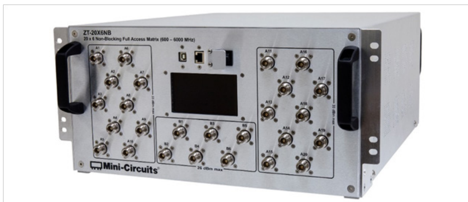
Figure 2: ZT-20X6NB in 6U height, 10-inch rack-mountable chassis.
