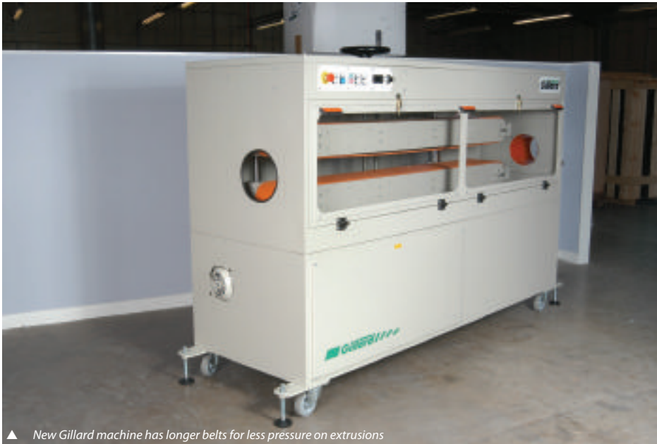
▲ New Gillard machine has longer belts for less pressure on extrusions
