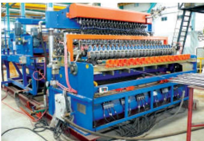
▲ Wire mesh welding line
