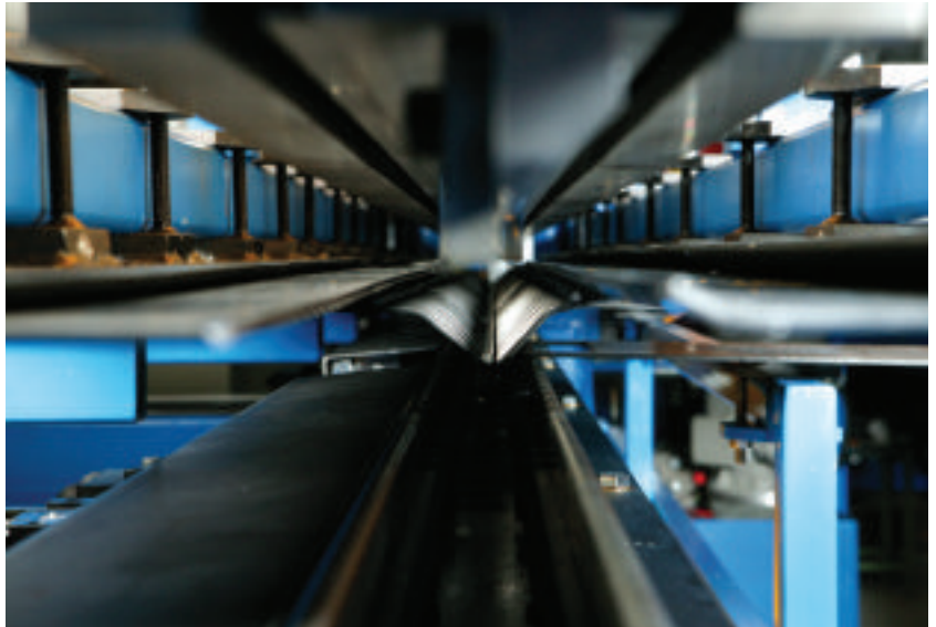
▲ Precision bending of fence mesh with Ravni equipment
