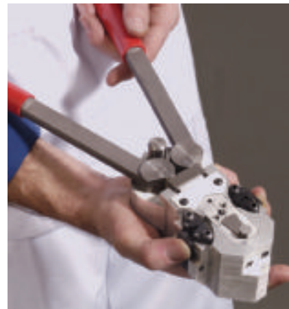
▲ The M30 hand held, manually operated cold welder has a capacity of 0.3mm to 1.8mm (0.0118" to 0.071") diameter copper/aluminium wire
