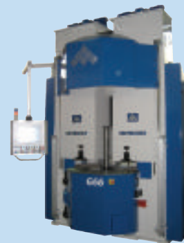
▲ Kamatech's G66TH1A with two working heads and central loading unit
