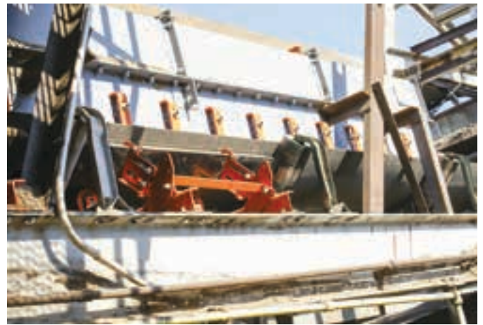
The cradles utilise 'double-life' slider bars for a flat, stable belt surface throughout the settling zone.
