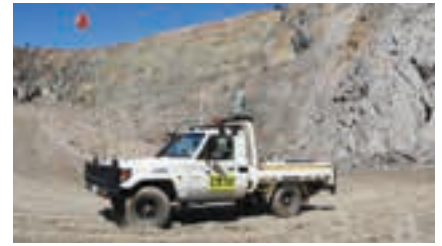
I-Site Drive continuously acquires data with a recommended I-Site laser scanner mounted on a moving vehicle.
