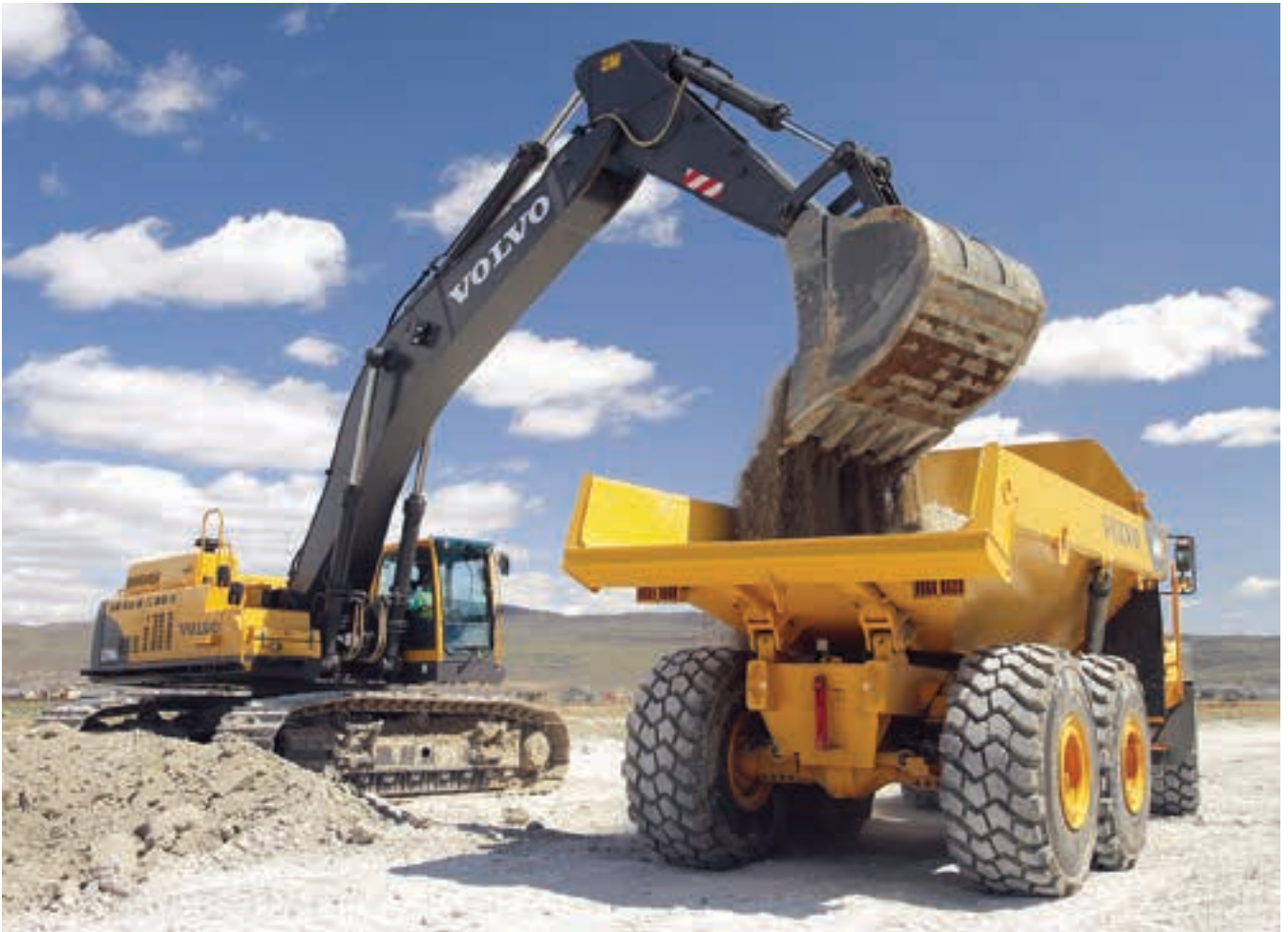
The Volvo EC700 excavator is well matched to the Volvo A40 articulated hauler.
