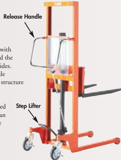
The release handle returns by spring tension, so in an emergency, the fork will stop lowering as soon as you release the handle.
