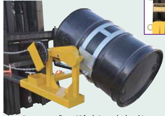
Rotates manually - a 15 ft. chain runs back to driver.
