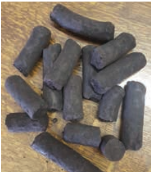
MAS has developed a pelletising process that transforms mineral fines and sludges into compressed pellets for sale or beneficiation.
