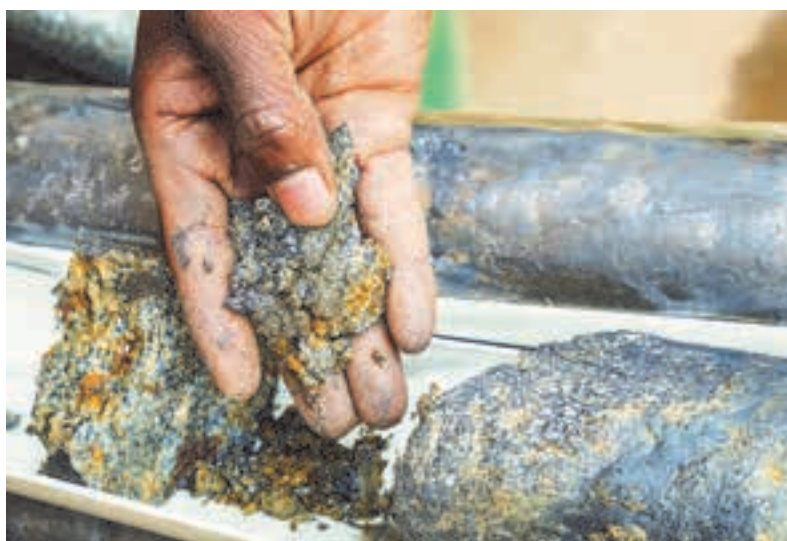
Soft, friable saprolite material from a diamond drill core sample at Malingunde.
