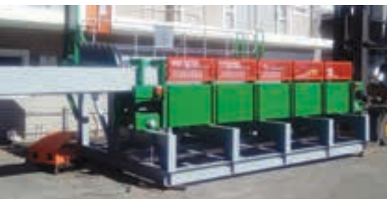
Front view of the rod charger showing erected boom.
