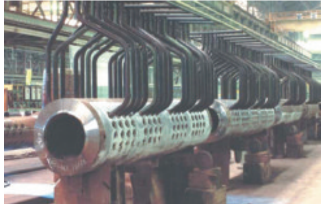
▲ Figure 2: Depiction of a typical header under fabrication at Mitsubishi Heavy Industries
