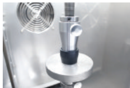
▲ In the hardness test: Rautitan PX compression sleeve stretch test
