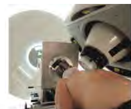
(b) Slit camera during patient treatment
