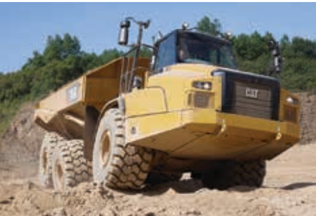
The Cat 745C has a newly designed dump body with a capacity (heaped SAE 2:1) of 25 m 3 and an increased payload of 41 tonnes.
