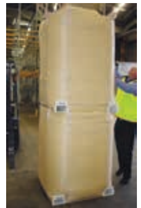
Tellap, which consists of a proprietary bulk bag and two strong integrated plastic sleeves, is lightweight, weighing only 5 kg, whereas a conventional wooden pallet can weigh up to 35 kg.
