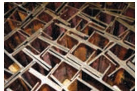
Stringer cleats which are used with Meshcape™ polyurethane screen decks.
