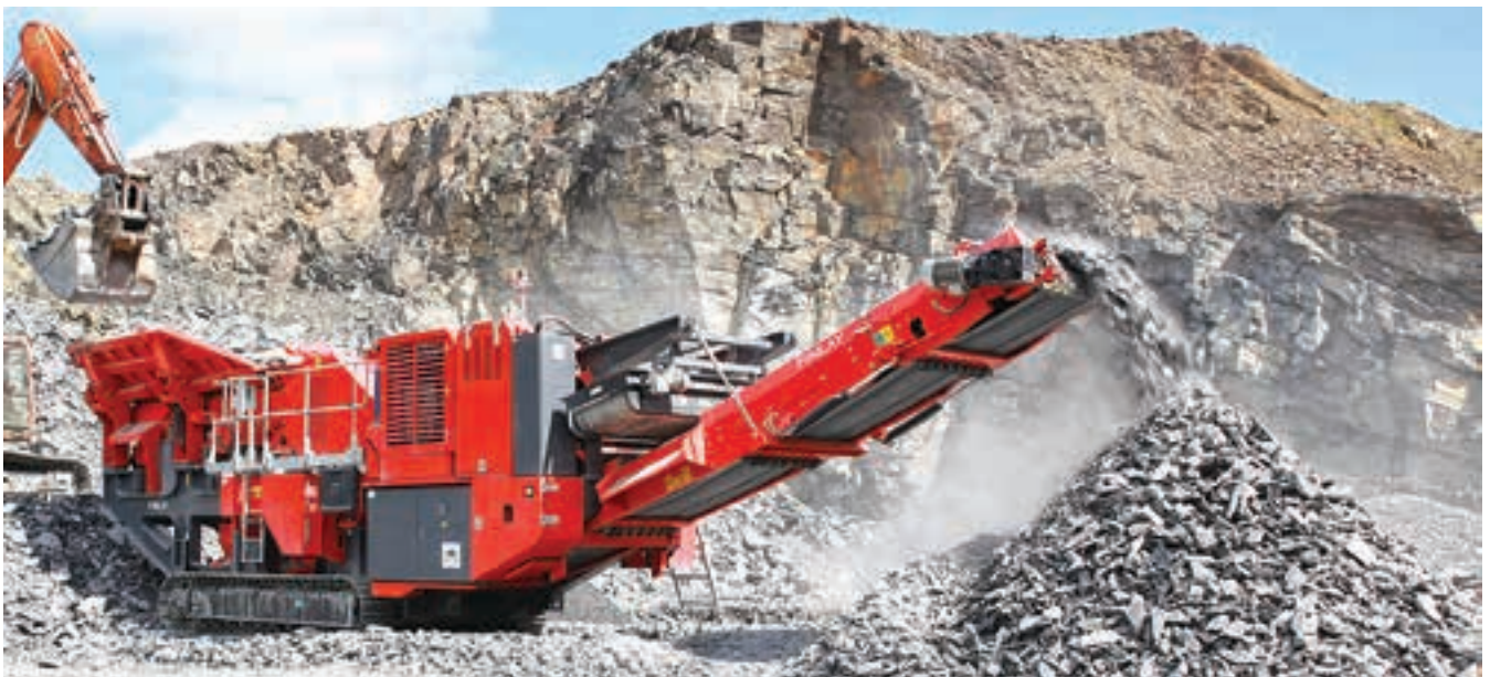
The J-1175 jaw crusher incorporates the robust JW42 high performance electrically driven single toggle jaw chamber and a heavy duty VGF feeder.
