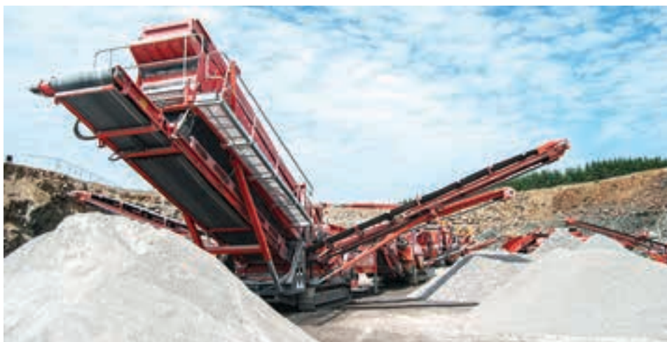
The 694+ dual power inclined screen features a large 6,1 m x 1,52 m triple deck inclined screen giving a total screening area of 28 m 2 .
