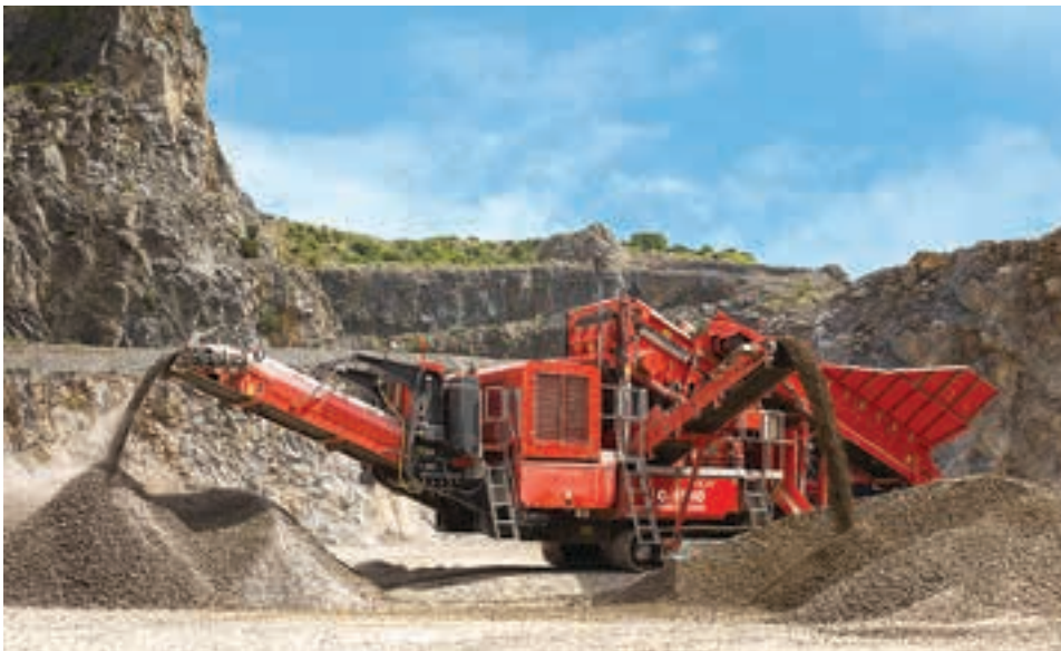
The C-1540 cone crusher makes use of the proven Terex® 1000 cone crusher with direct electric drive, automatic tramp relief and hydraulic closed side setting (CSS) adjustment.
