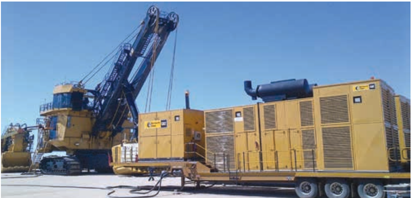
The Cat C175 diesel engine motivator in the foreground was designed and built by Barloworld Power to power up the Cat 7495 electric rope shovel in the background for movement around the mine.
