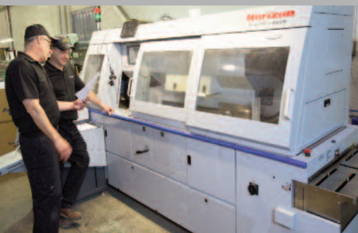
The Standard Horizon BQ-470 Perfect Binder was installed and operational in under a day.
