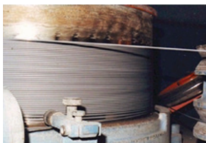
▲ Anti-wear high-melting coat on 0.85% C descaled wire
