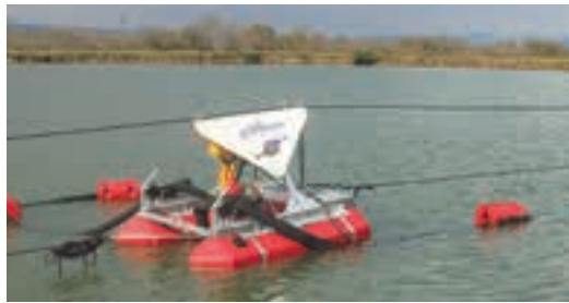
Left: The innovative SlurrySucker Dredge Unit is capable of extracting high tonnages of silt and built-up sediments at a fraction of the cost required to shut down downstream and upstream storage facilities.
