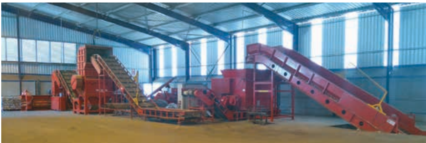
A view of the RDF processing plant for 'fluff'. Non-recyclable plastic waste is loaded onto a feeding platform before being passed through a primary and then a secondary shredder. The fluff is then bailed ready for transportation to a power station, kiln or industrial burner.
