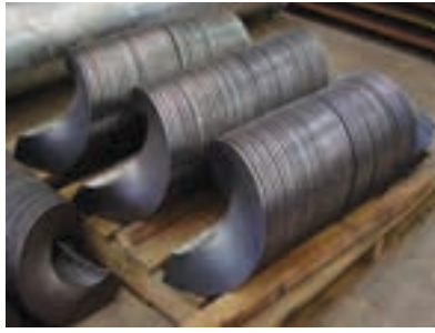
Bruton Spiralfight's new state-of-the-art forming press allows the company to offer diverse materials such as Hardex™ in various flight sizes; from 1 200 mm outside diameter in thicknesses from 16 mm to 25 mm.
