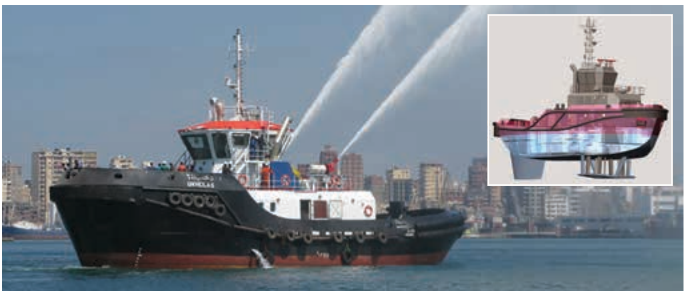
Voith Water Tractors with Voith Schneider propellers have been deployed at the Port of Alexandria since 1989.
