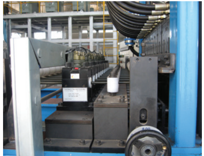
Junction detection on copper alloy double wall tubes
