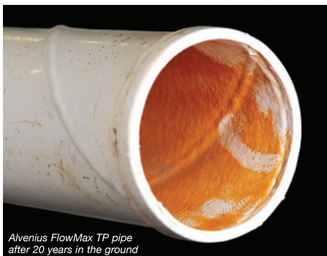
The pipe, after being cleaned with high-pressure water, shows no defects
