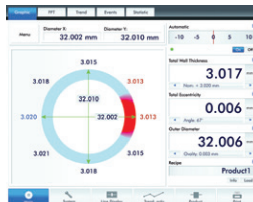
Integrated in the extrusion line the X-ray measuring system X-RAY 6000 measures the wall thickness, eccentricity, the inner and outer diameter and the ovality of hoses and tubes
