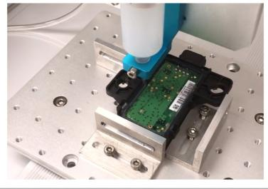
Even complex program patterns can be developed quickly using the simple point to point teach pendant. Dispense adhesive direct from syringes or optional metering valves and pressure pots. With fast indexing speeds, high accuracy and simple programming; robots are an ideal solution for most dispensing applications in a 200mm x 200mm work area. CE approved. Advanced features include work pattern array copy, end of cycle brush or wipe mode and slope dispensing.
