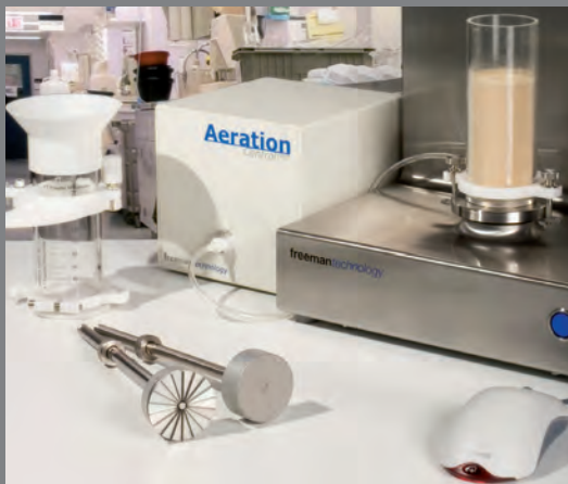
Air in Aeration test
