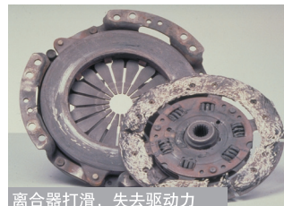
离合器打滑, 失去驱动力 Slipping and Loss of Drive
