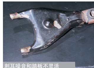
刺耳噪声和踏板不灵活 Grating Noise and Stiff Pedal
