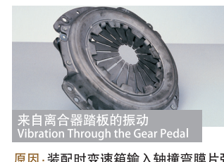
更换离合器后发抖 Juddering After Changing the Clutch
