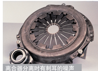
离合器分离时有刺耳的噪声 Harsh Noise on Declutching
