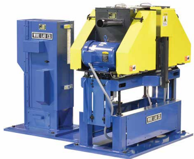
▲ The 1250 automatic brush descaling system
