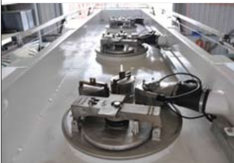
Tank walkway showing hatch systems, vapour recovery fittings and pneumatic safety railing.
