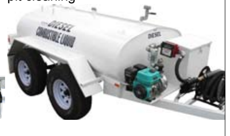
Conventional diesel trailers in 1k, 2k and 3500L versions. Reg'ble & unreg'ble with range of pumpsets
