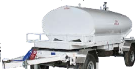
Dangerous Goods Approved trailers for Class 3 Flammables - Petrol, AvGas, Jet-A1.
