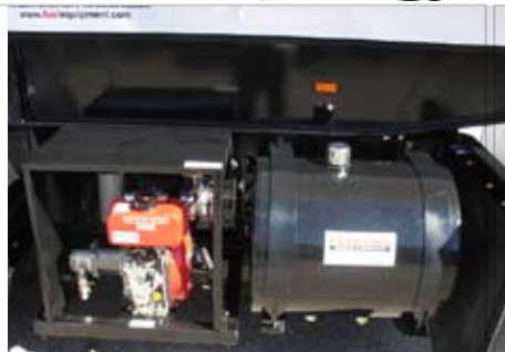
Yanmar diesel engine-powered hydraulic power pack makes this vehicle a complete stand-alone fuelling system.
