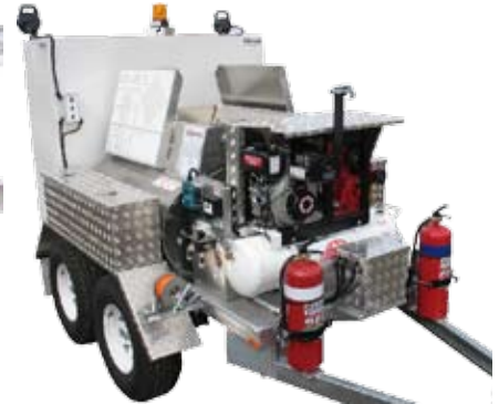
Dangerous Goods Approved trailers for Class 3 Flammables - Petrol, AvGas, Jet-A1.
