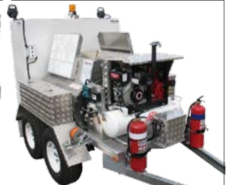
Dangerous Goods Approved trailers for Class 3 Aviation fuel quality test & hydrant pit cleaning
