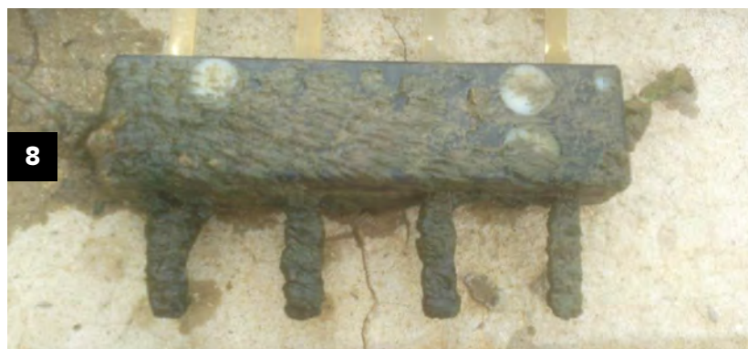
Figure 1: Block one of the BOMM indicating the positions of the corrosion coupons (red).
