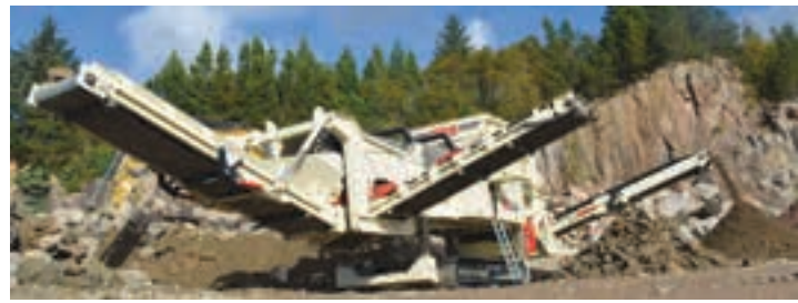
MDS M515 trommel screening primary blast material up to 800 mm.
