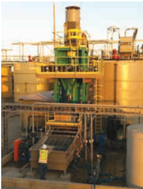
This VXP2500 in Zimbabwe was the first of the updated VXP2500 mill series.
