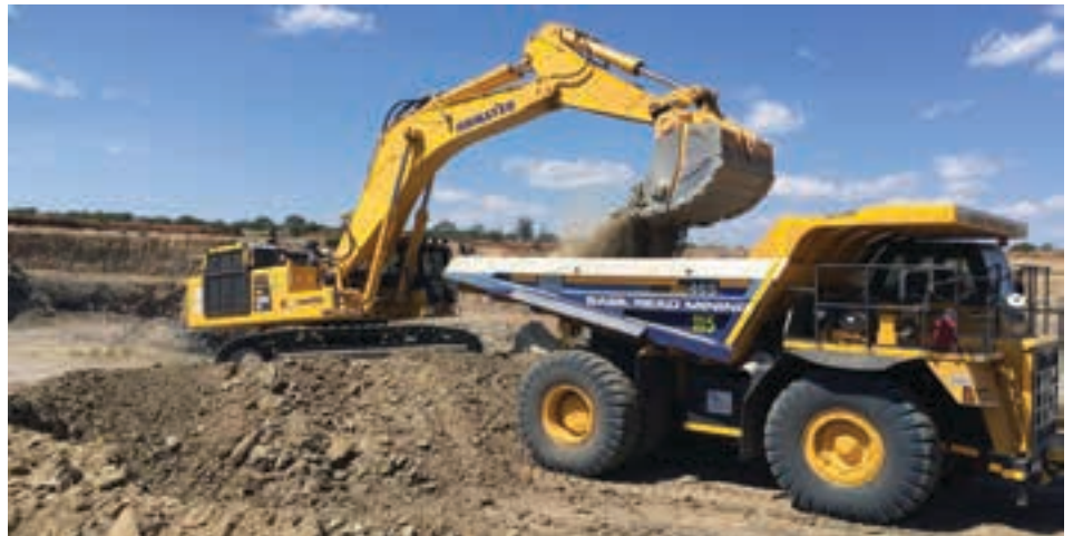
First kimberlite ore being mined and hauled from the K3 pit at Lerala (photo: KDL).
