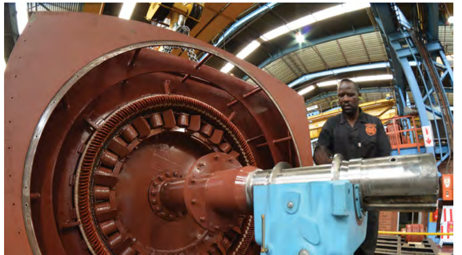
Alpheus Mtshali, from Marthinusen & Coutts, is pictured with the 1 586 kW 1875 rpm, 3 300 V, 278 A stator.
