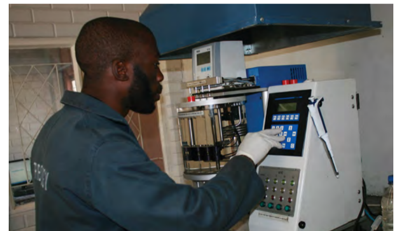
Admire Katanda, lab technician at WearCheck Zim operates a viscometer.
