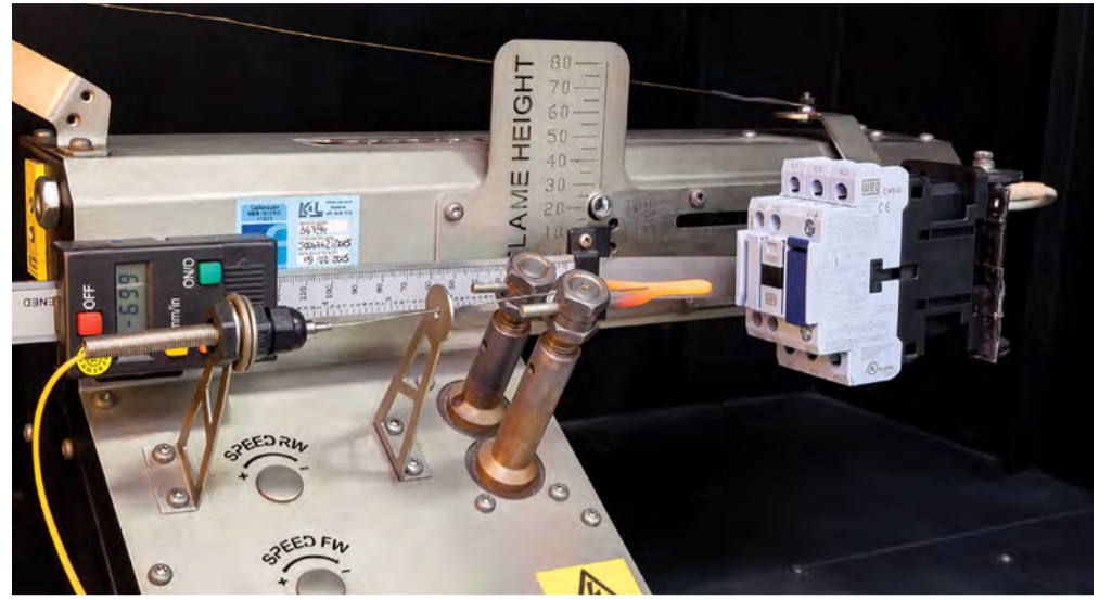
The WEG CWB range of contactors undergoing a glow wire flammability test according to IEC 60695-2-11.
