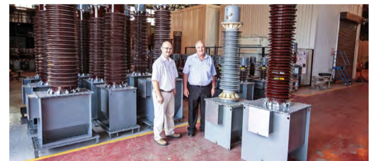
Nick de Beer (product manager, instrument transformers) and Etienne Venter (design engineer, voltage transformers) of ACTOM High Voltage Equipment stand next to a compact 132 kV voltage transformer, which is substantially smaller than the conventional units around it, as the picture shows.
