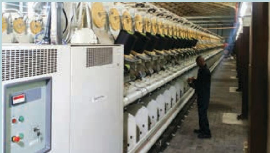
The newly installed yarn twisting machines at the PFE Extrusion factory in Hammarsdale.
