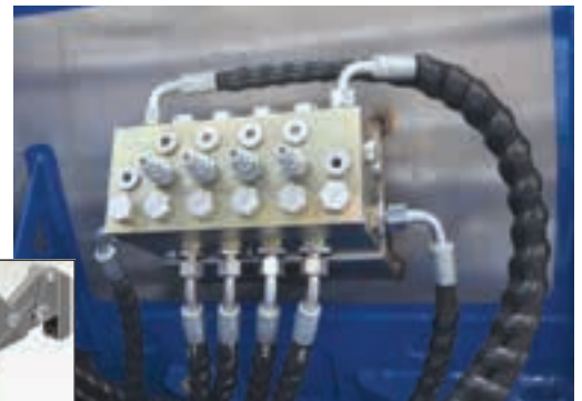
The hydraulic control system, with its manifold block and Sun Hydraulics "kick-down" cartridge valves, is designed, built and manufactured in South Africa by Axiom Hydraulics. Left: A SolidWorks rendering of the hydraulic clamping mechanism.
