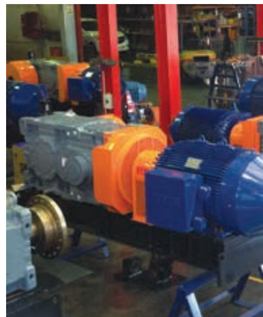
As well as servicing, all SEW-Eurodrive branches are being equipped to enable them to produce final drive assemblies – fitting motors, gearboxes, couplings and drives onto base-plates for delivery to site as a single unit.
