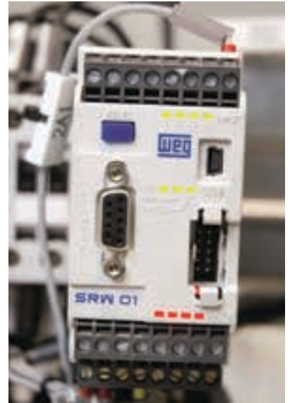
Designed for use with power supplies from 24 to 220 V ac/dc, the WEG SRW01 has a facility, if selected, to monitor voltage up to 690 V ac and measures current from 0.25 A up to 840 A.
