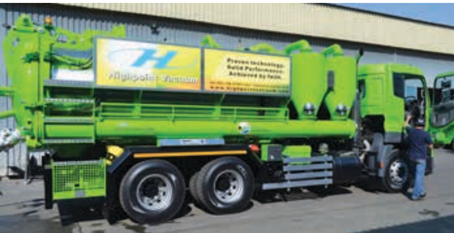
Highpoint Vacuum's 1000-PDB dry bulk vehicles use positive displacements roots blower-type vacuum pumps.
