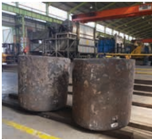
With a height of 850 mm, these forging are two of the 43 large nozzle components ordered by a South African customer for a pressure vessel application.
