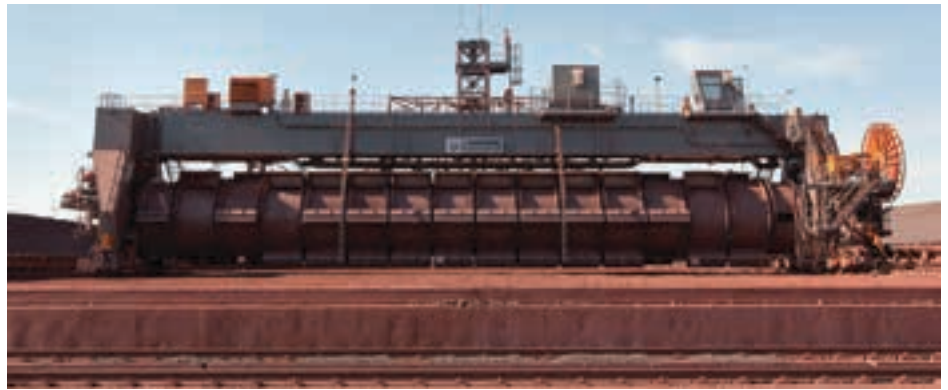
Currently being commissioned, a new thyssenkrupp drum reclaimer for an iron ore mine in the Northern Cape mine. The single shell design makes these new machines less complicated and less expensive to fabricate, while finite element analysis techniques enable optimisation of the shell thickness to best suit the application.
