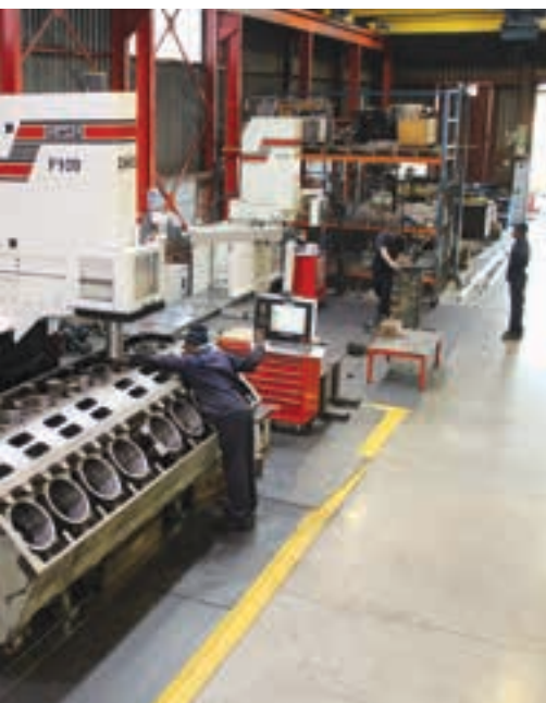
Above: This unit, one of only 11 operating worldwide, provides consistent accuracy levels and has the capacity to handle 6.5 m blocks. Left: Metric Automotive Engineering’s facility in Johannesburg, Gauteng, also features a three-axis computer numerical controlled machining centre.
