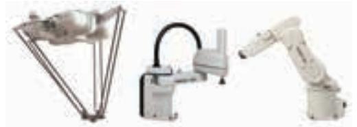
Omron has released 49 new best-in-class robots, including models from three robot families, from left: Delta (Quattro); SCARA (eCobra); and Articulated (Viper).
