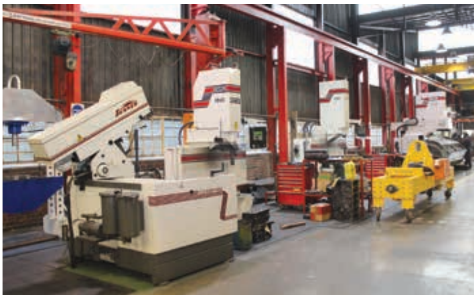
Above: This unit, one of only 11 operating worldwide, provides consistent accuracy levels and has the capacity to handle 6.5 m blocks. Left: Metric Automotive Engineering’s facility in Johannesburg, Gauteng, also features a three-axis computer numerical controlled machining centre.
