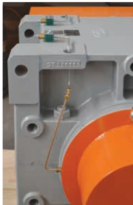
Right: In addition to the pony-drives, the Bonfiglioli HDO 130 units were customised with additional piping and lubrication points to facilitate easy maintenance once installed. Rigid flange couplings on the low speed shafts, together with safety guards are also fitted.
