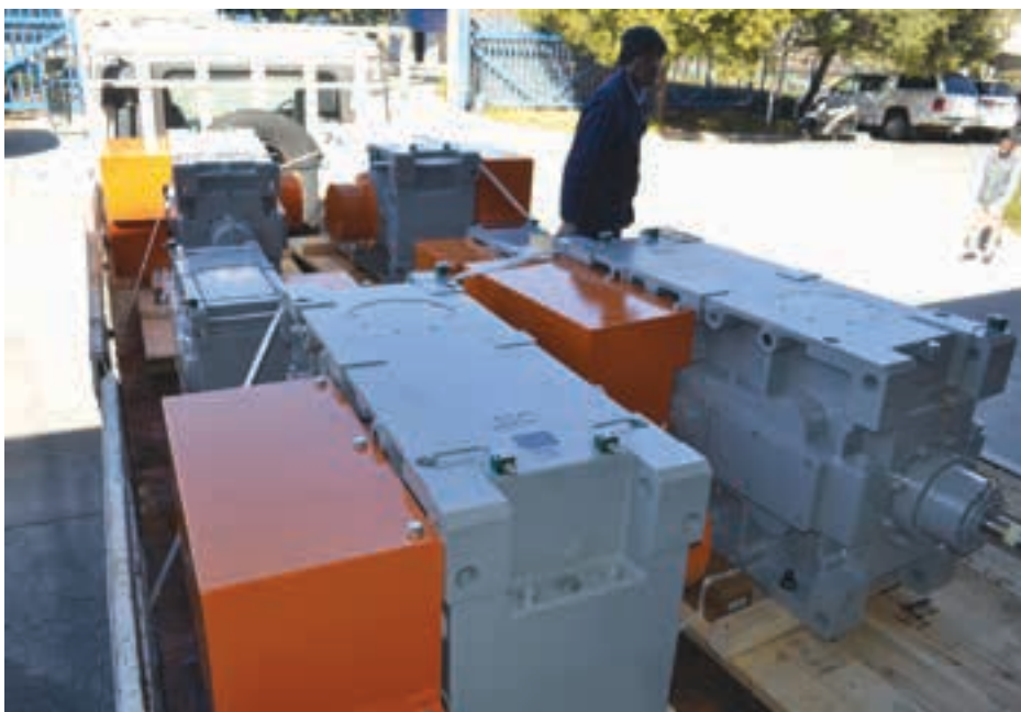
Some of the final batch of Bonfiglioli HDO 140s along with HDO 100s being loaded onto one of the trucks for delivery to the client.
