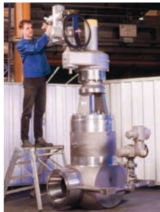
KSB's valve repair workshop is able to undertake all repairs and refurbishment of large-scale and complex valves, including high-pressure steam valves.
