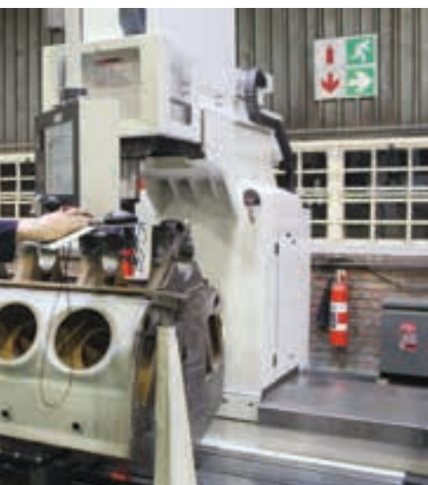
Left: Metric Automotive Engineering operates a crankshaft-grinding machine capable of grinding shafts of up to 4.7 m long and with weights of up to 5.0 t. Centre: The company operates the only CNC machining centre of its kind in Africa, capable of line boring, surfacing and blue-printing blocks up to 6.0 m in length. Right: A major differentiator for Metric Automotive Engineering is its ongoing investment in the dedicated equipment that is needed to provide a thorough and quality remanufacturing service.
