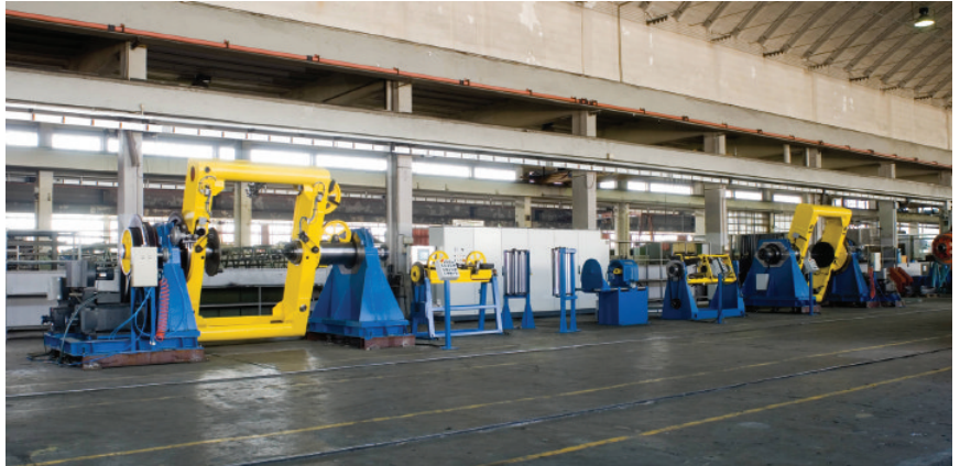
▲ Cortinovis Machinery's Monotorsion armouring and screening machine
