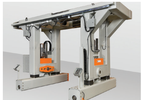
▲ GTU-100A 1440D x 100W gantry system from Tulsa Power
