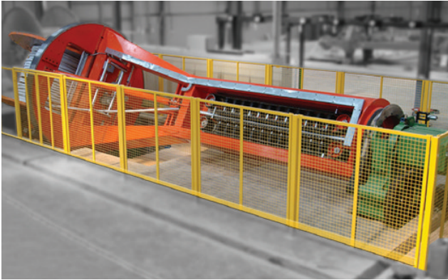
▲ OM Lesmo's drum twister for power cable
