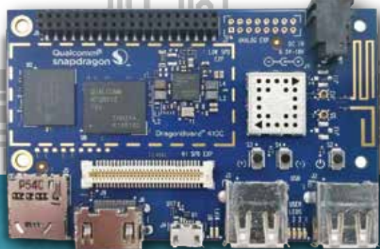
Dragonboard410C based on Qualcomm Snapdragon410E
