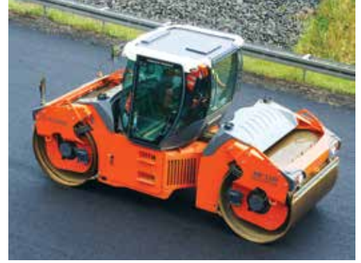
A HAMM HD+ 120i OV tandem roller compacting the surface course of a busy highway.
