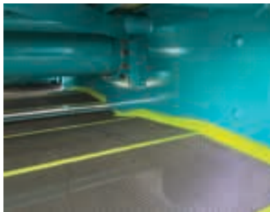
Flex-Mat 3 Series D high frequency tension mats with side seals to prevent contamination of the undersize.
