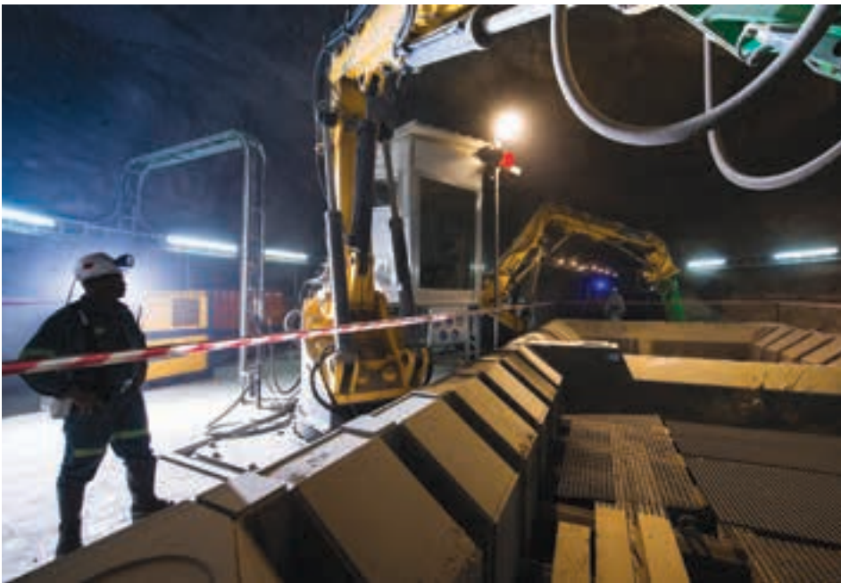
Tips and impact breakers on 839 level – the new production/extraction level for Cullinan's C-Cut project (photo: Petra Diamonds).
