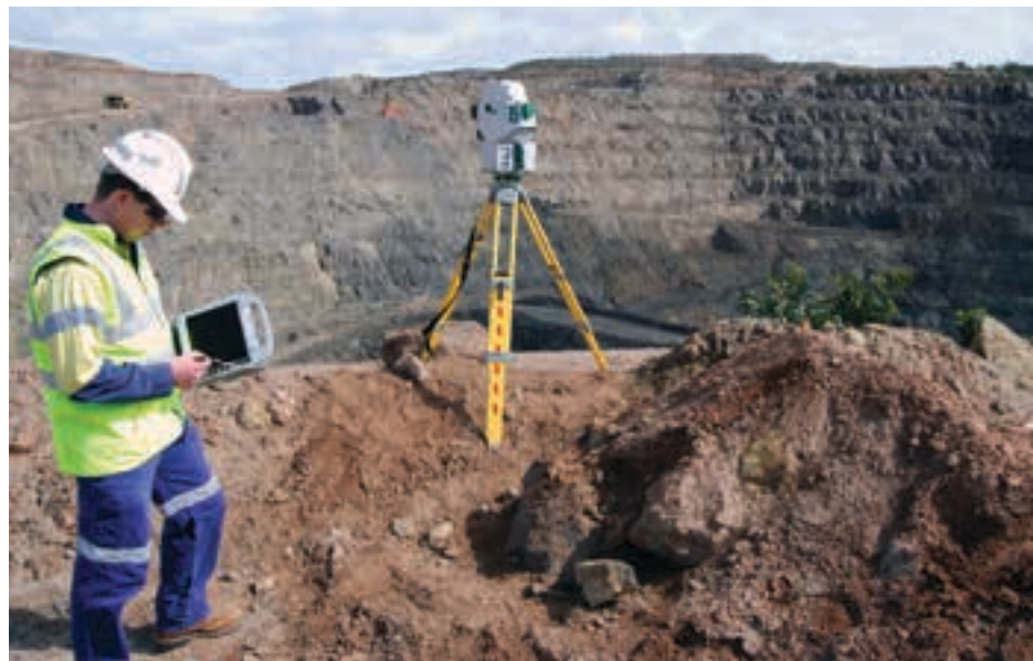
Maptek's I-Site 8800 laser scanner. It can be used in open-pit or underground mining applications.
