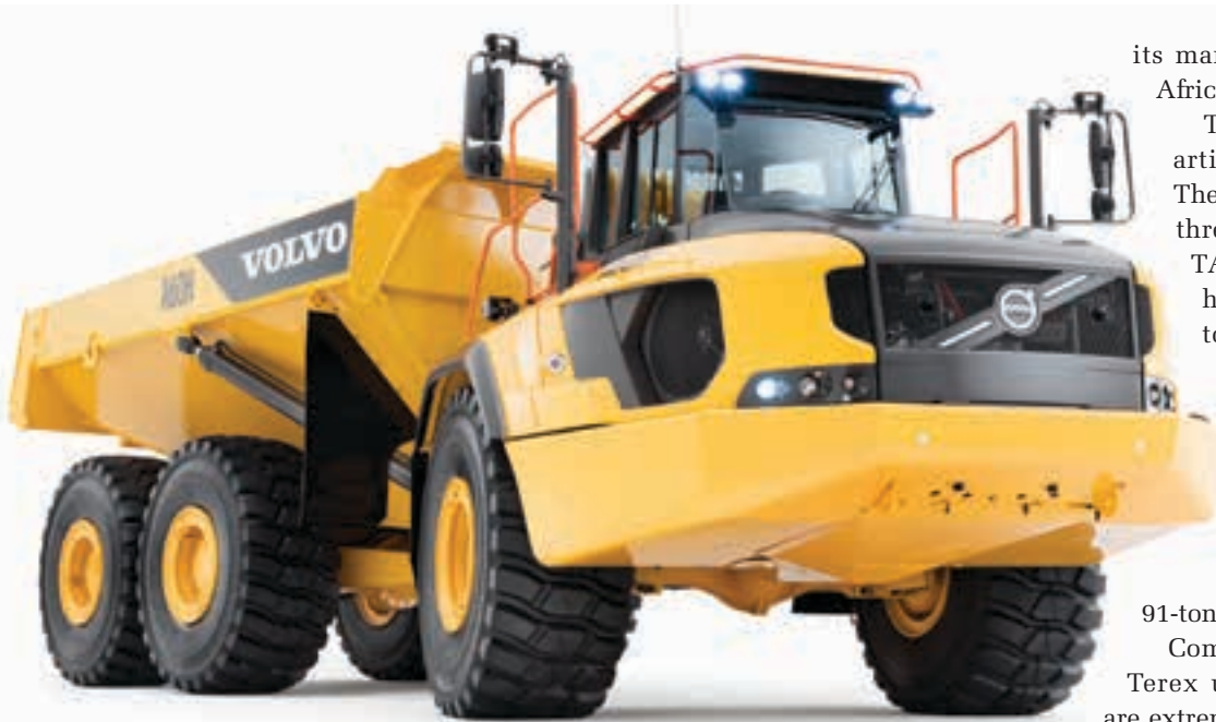
The payload of the A60H is 61 short tons or 55 metric tons (tonnes).
