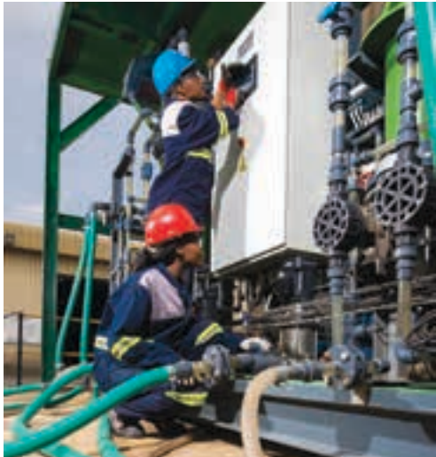
Multotec's 1 m 3 /h DeSALx test rig that is used to do on site testwork at customer sites.
