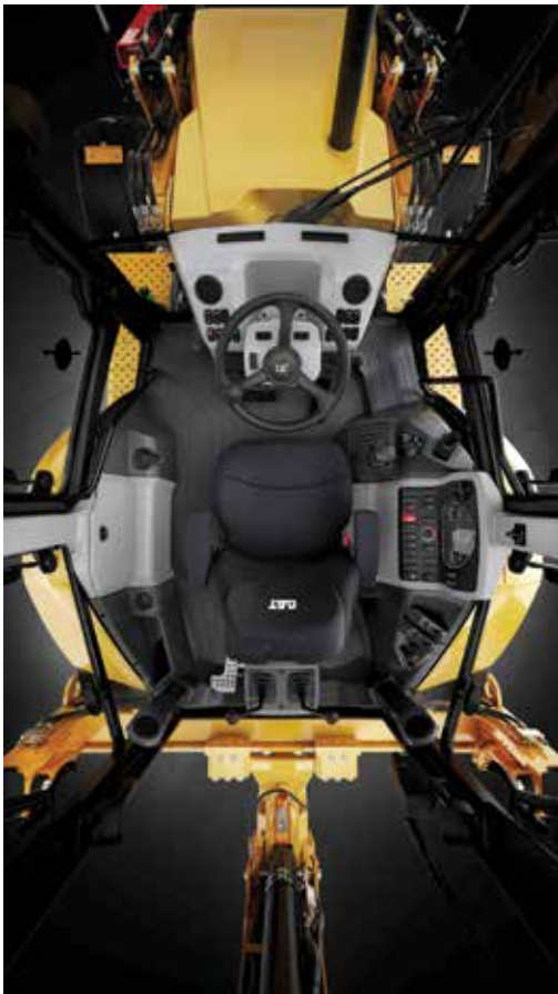
In-cab, a new LCD display provides the information needed to monitor machine performance. New switches feature improved back lighting for easy use in all ambient-light conditions, and longer-life LED rear lights are now standard. (This cab view shows the machine specified with mechanical controls.)
