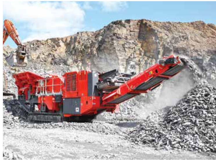
The dual-powered Finlay J-1175 jaw crusher offers operators flexible power operations.
