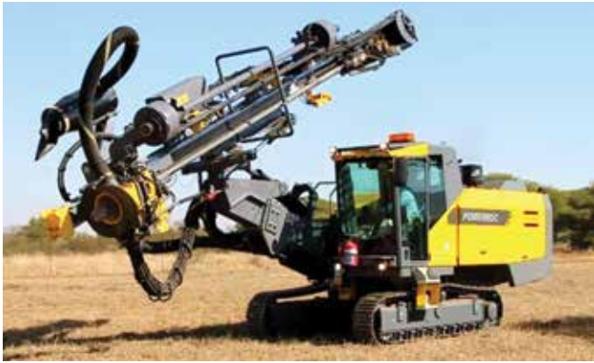
The DCT 200 dust collector provides strong dust suction capacity and excellent dust suppression. There are 20 filter elements with a total filter area of 20 m 2 .
