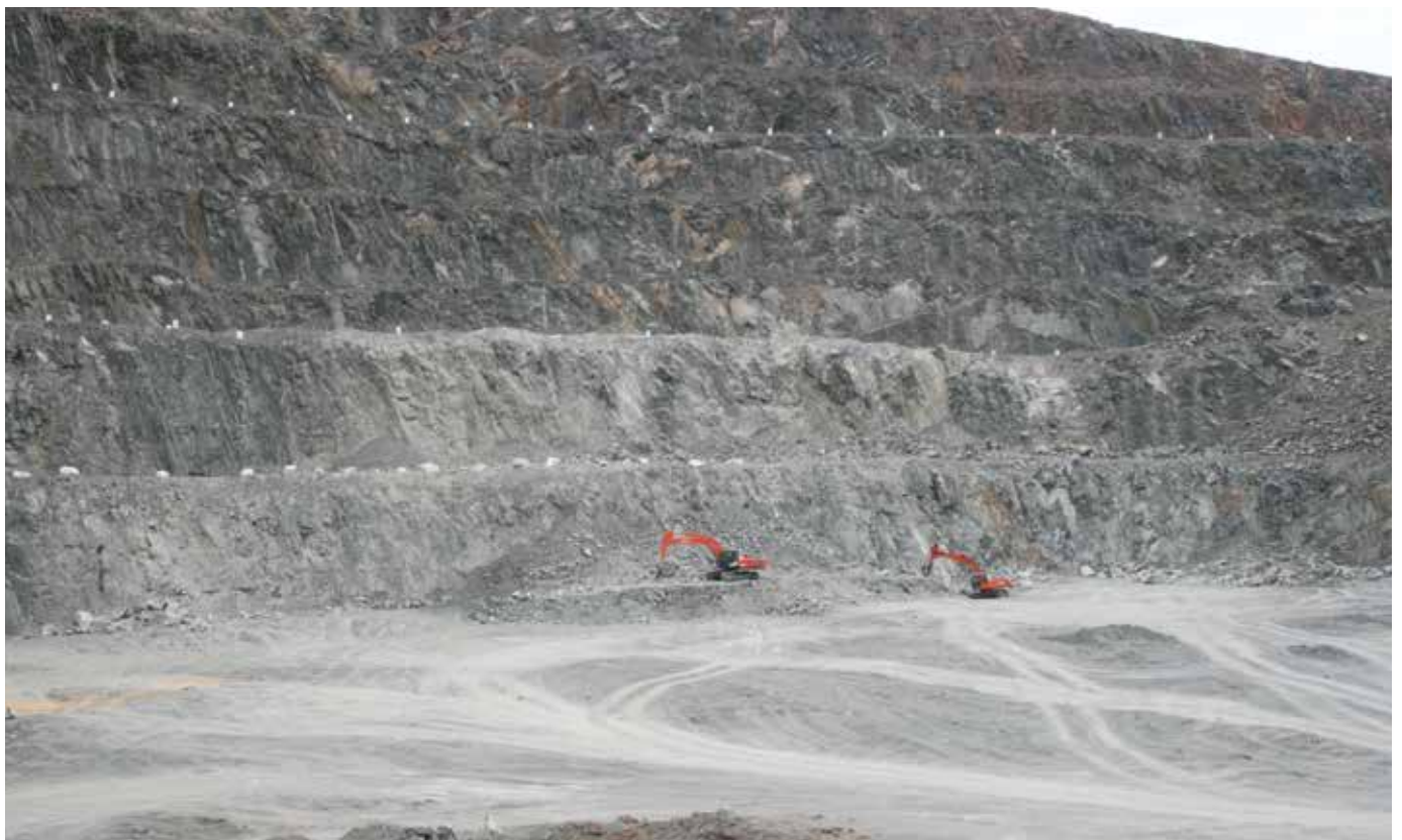
The mine is carrying out the pre-split lines on the benches with future development being on the floor.
