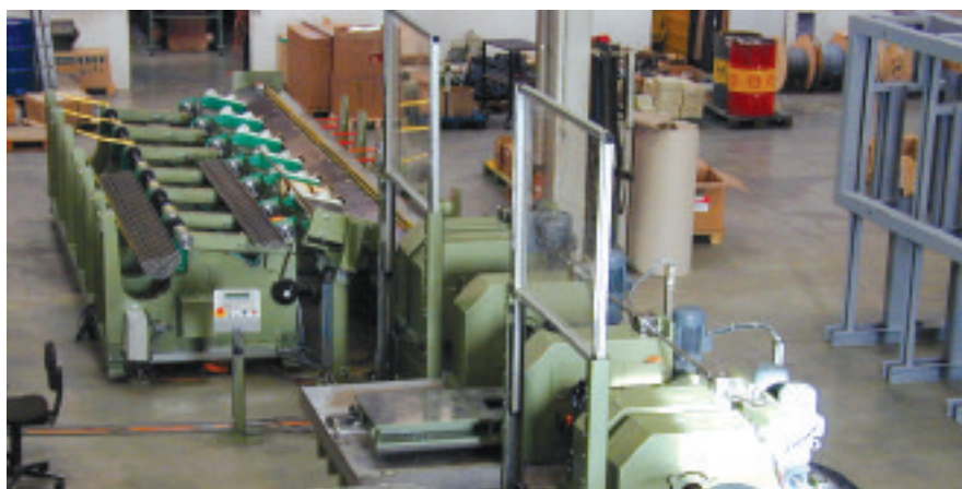
○ sema Systemtechnik testing line for round and hexagonal material
