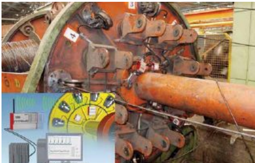
▲ A multi-stage planetary strander that was upgraded with FMS Tension Monitoring System RTMX42
