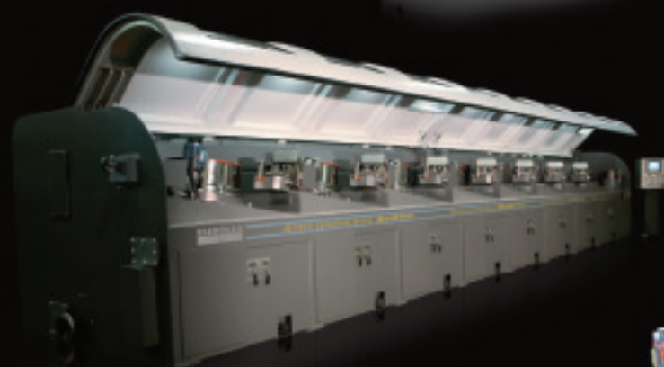
Cold rolling lines with cassettes
