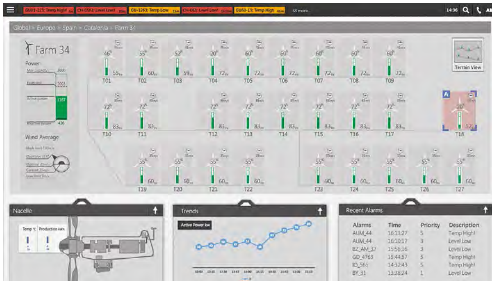
Figure 1: Farm view with one tower selected, showing recent alarm history and power output
