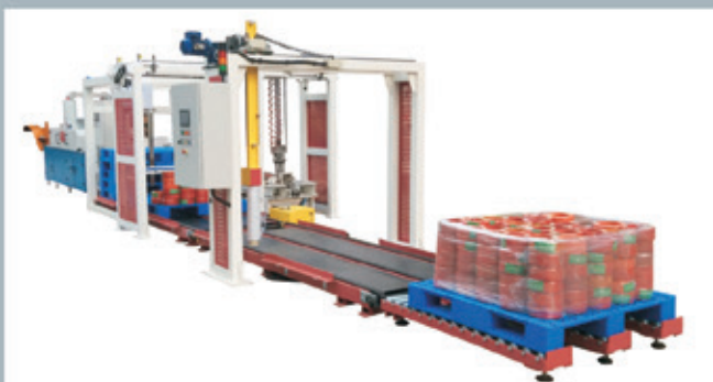
Auto coiling and stacking line
