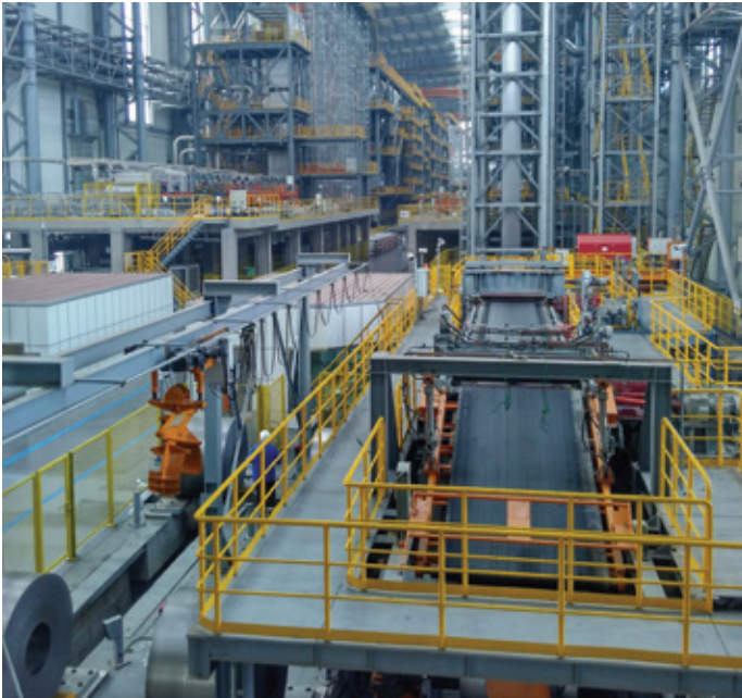
○ The existing galvanising line supplied by Primetals Technologies in the cold rolling mill of Tangshan Iron and Steel Group Co Ltd. The company has now ordered two further lines
