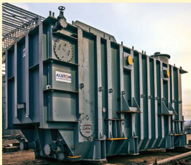
○ First transformer for the Champa-Kurukshetra UHVDC phase 1 link
