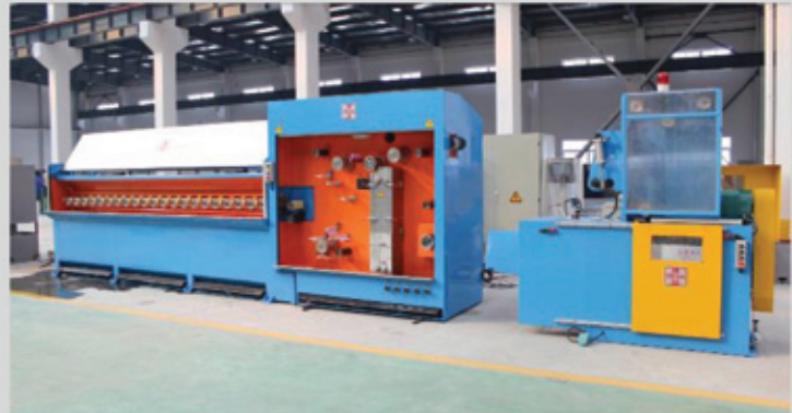
Multi-wire drawing machine with continuous annealer
