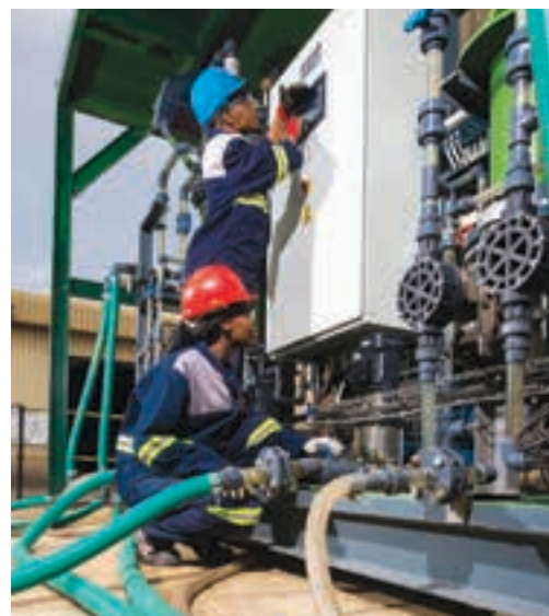
Multotec's 1.0 m 3 /h DeSALx test rig used to do on site test work at customer sites.
