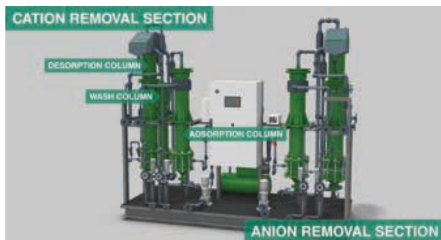
Multotec's dual stage continuous desalination process consists of cation removal followed by anion removal, with each section consisting of three columns.
