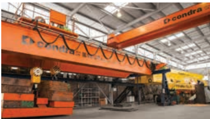
One of Exxaro's three cranes for Grootegeeluk Coal Mine undergoing load testing at Condra's Germiston factory.
