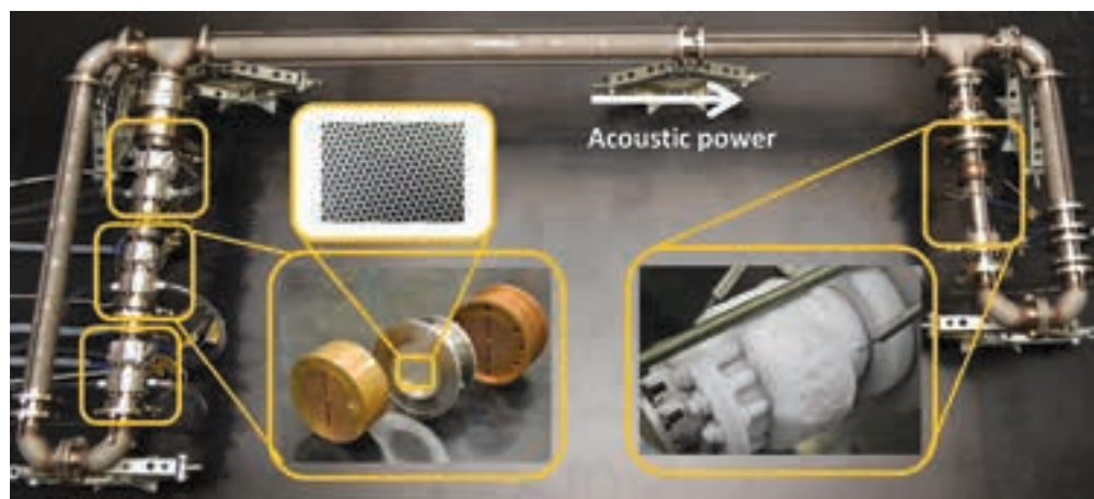
The double loop TWTR consists of three etched stainless steel mesh regenerators installed within the prime mover loop (left). This creates acoustic waves that drives the refrigerator loop (right).
