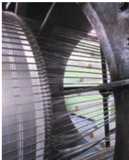
The wedge wire machine long wire feed assembly.
