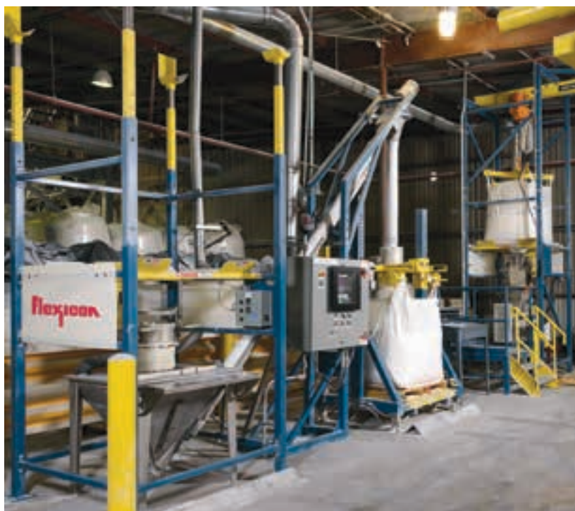
Two bulk bag dischargers, a flexible screw conveyor, a bulk bag filler and programmable controls allow re-bagging of PVC modifiers into bulk bags of three sizes and 23 kg sacks, efficiently and dust-free.
