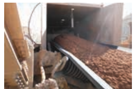
Weba Chute Systems incorporate a supertube or cascade scenario with material running on material.
