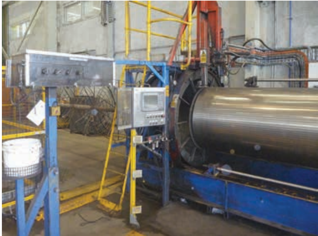
The new wedge wire machine recently commissioned by FLSmidth in its Edenvale facility.
