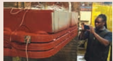
Marthinusen & Coutts' rotating machines design engineer, David Motloun, records photographic evidence of tests on one of the enormous gearless mill drive rotor poles recently refurbished by the company.
