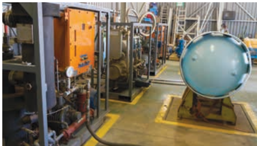
The ZUGIBEAST is a high-speed decontamination unit used to extract contaminants from refrigerants.
