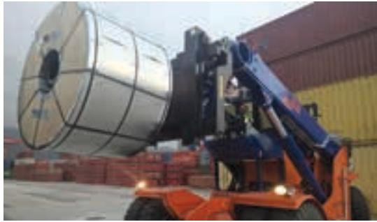
The Meclift range of heavy lifting equipment, available exclusively in South Africa from materials handling specialists, BLT SA, is available with a coil ram attachment for handling steel coils.
