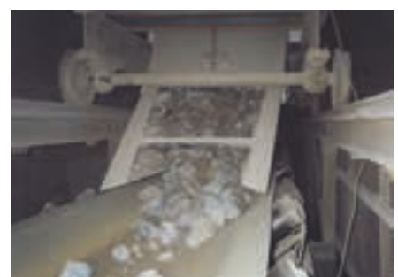
Weba Chute Systems are engineered to control the materials’ flow.
