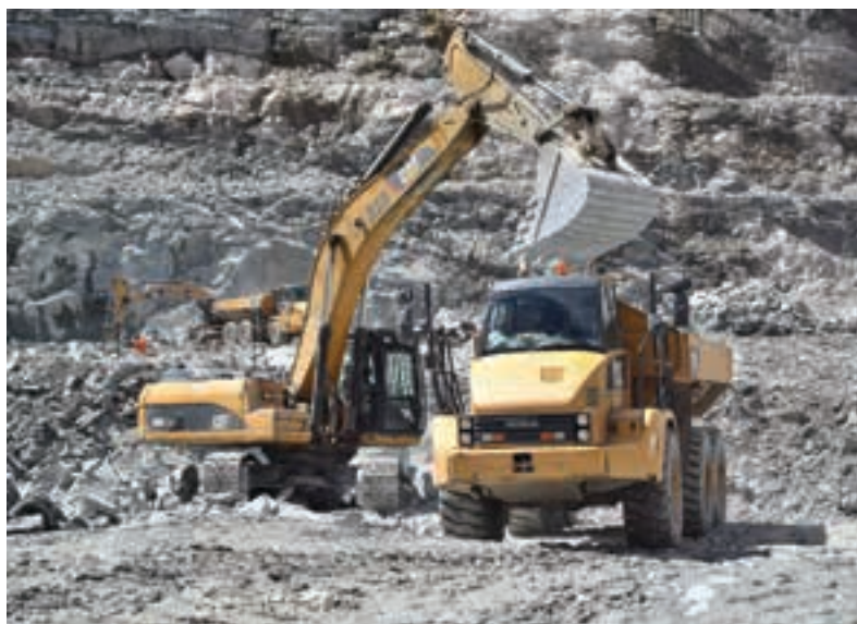
A Cat 336D excavator loads a Cat 730C ADT. Kagem's mining fleet is modern and well maintained.
