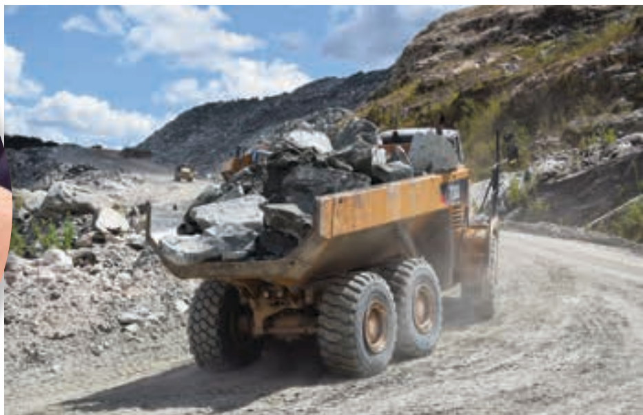
A Cat 730C articulated dump truck (ADT) hauls its load out of the pit. ADTs are preferred to rigid trucks at Kagem due to their better manoeuvrability.
