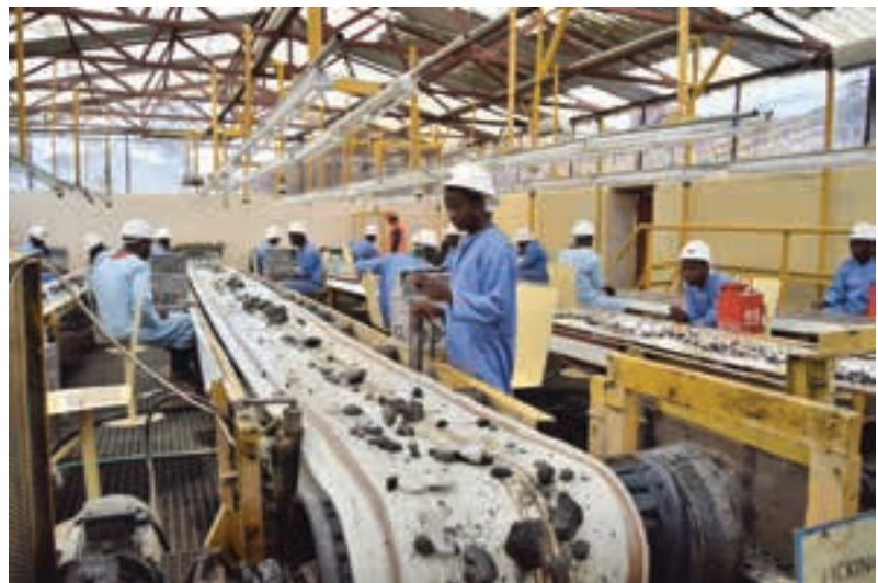
The picking belt facility, which is part of the washing plant, where the emerald crystals are picked out by hand from a series of picking belts.
