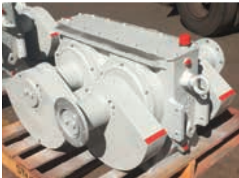
Specialist vibrating equipment supplier Joest South Africa has introduced a new exciter gearbox.
