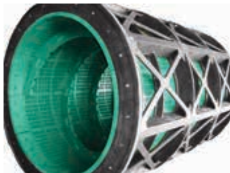
A SAG mill trommel frame with cast polyurethane screen panels and a pinless fastening system.
