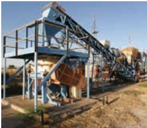
The 10 t/h DMS plant acquired by Tsodilo Resources for the BK16 project.
