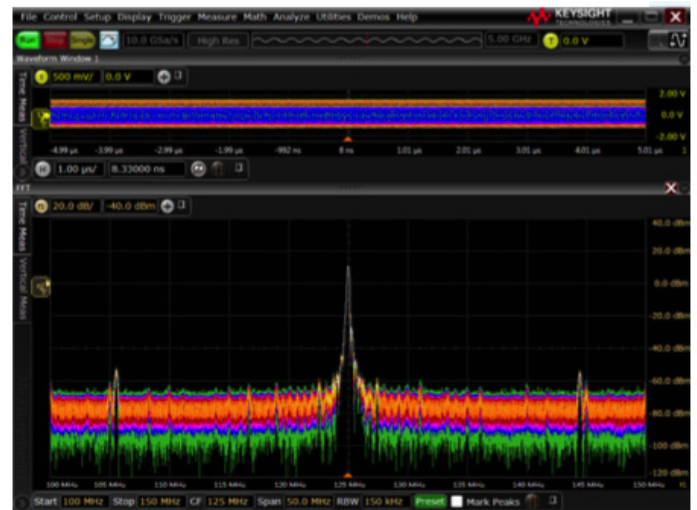
Figure 8: The 7MHz clock sidebands have been eliminated by inserting the series resistor between the regulator and the clock, damping the PCB resonance.
