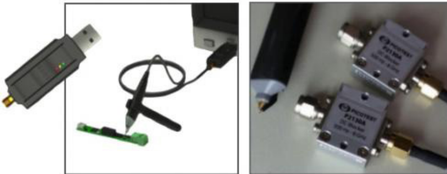
Figure 4: Simple but effective tools support PDN interrogation and clock jitter assessment. These include a J2150A harmonic comb broadband signal generator (left) along with 1-port (center) and 2-port bi-directional 50Ω passive probes and DC blockers (left).
