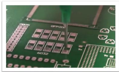
Even complex program patterns can be developed quickly using the simple point to point teach pendant. Dispense adhesive direct from syringes or optional metering valves and pressure pots. With fast indexing speeds, high accuracy and simple programming; robots are an ideal solution for most dispensing applications in a 300mm x 300mm work area. CE approved. Advanced features include work pattern array copy, end of cycle brush or wipe mode and slope dispensing.
