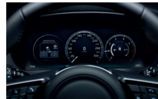
12.3 inch Instrument Panel Display with virtual dials
