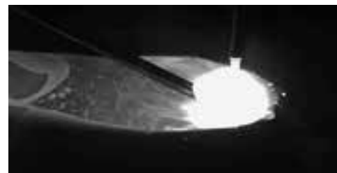
Figure 5: A photograph of the GMAW arc and the hot wire entering the weld pool.
