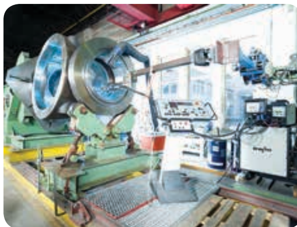
Figure 8: The GMAW hot wire welding system in use.
