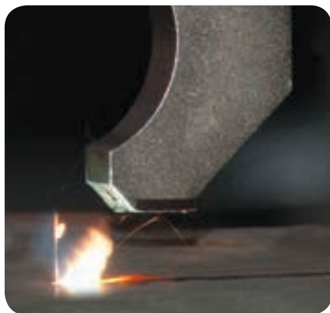
Nexelia’s Nozzle-Jet consists of two independent gas circuits: The first argon stream blows any plasma or fume clear of the laser’s beam line, while the second ‘diffuser’ shields the hot weld seam.
