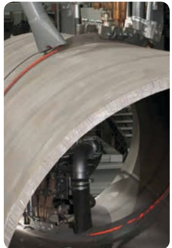
The advantages of SAW over other welding processes include: high deposition rates; typically deep penetration; high operating factors, due to the mechanised nature of the process; and low hydrogen levels in deposited weld metal.
