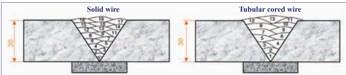
A 30 mm V butt joint was filled using 19 solid-wire SAW beads, while only 13 were required when using Fluxocord 31 HD.
