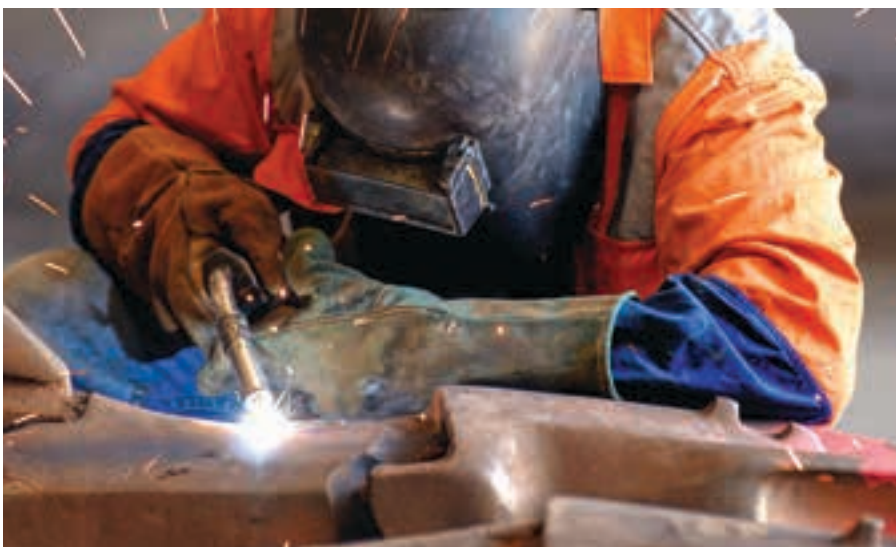
With the Fluxofil HD range of tubular cored wires, filling factors have been further increased.
