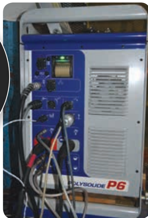
The heart of the orbital system for this application is Polysoude’s P6 TIG welding power source with its integral orbital welding control system.
