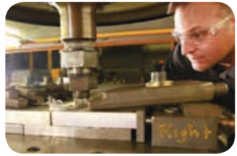
Friction stir welding increases the ability to produce products with a wider array of alloys.
