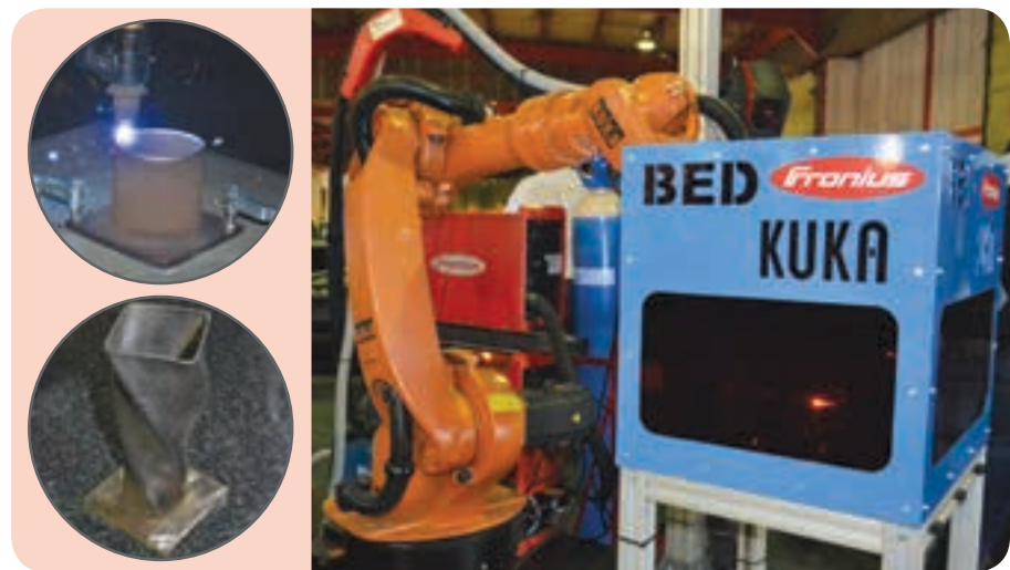
At Machine Tools Africa 2017, an industrial robot and Fronius' CMT welding process was demonstrated manufacturing a 3D-printed steel vase.
