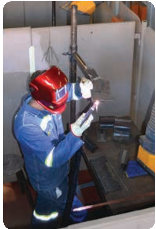
A trainee practising his gas-tungsten arc (GTAW) skills in the SAIW welding school.
