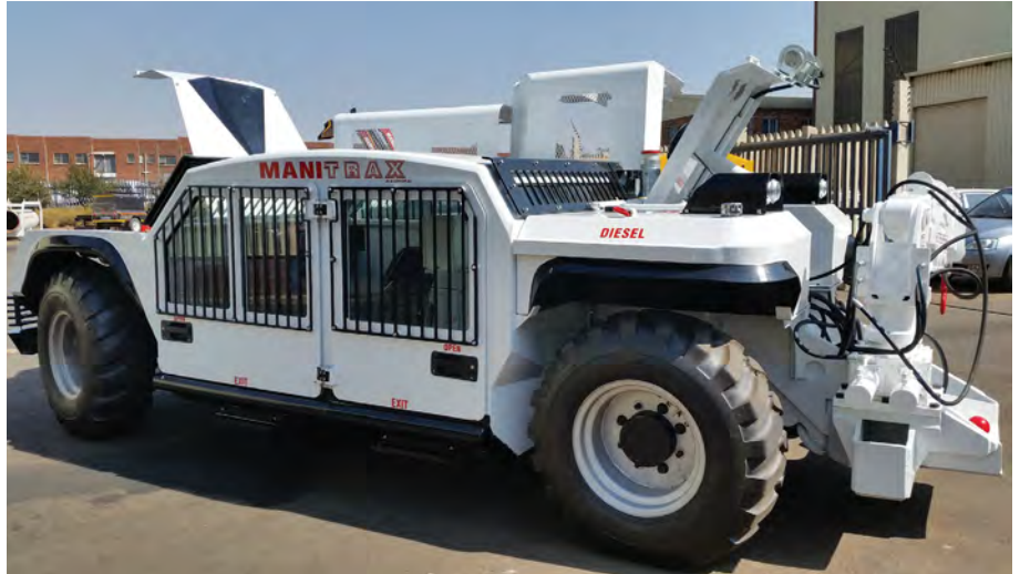
Manitou Southern Africa will show its 35 t tow tractor designed for underground use, but can also be deployed in aboveground mining applications.
