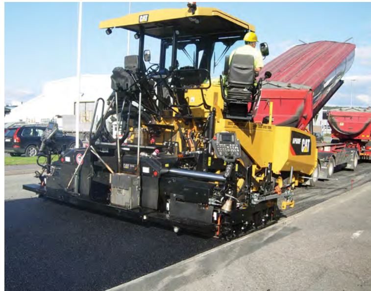
Caterpillar's AP655F is a rubber track paver equipped the exclusive Mobil-Trac undercarriage.
