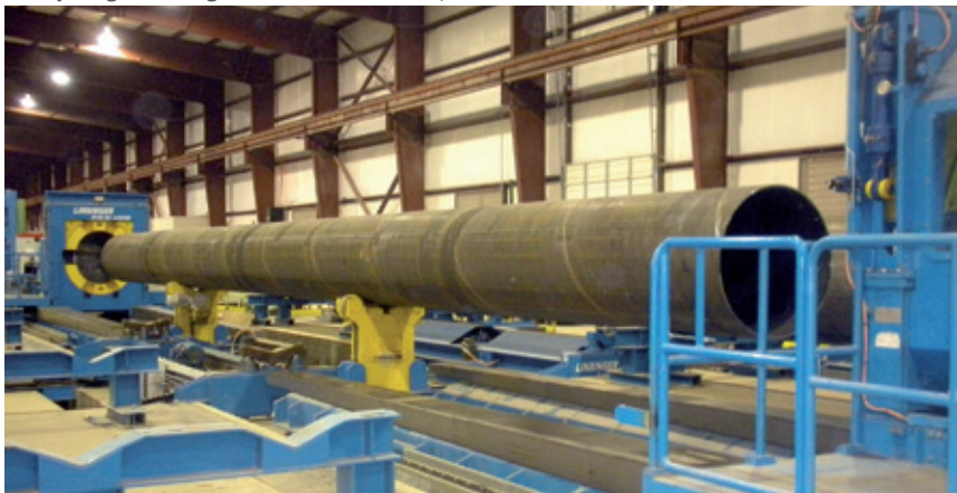
Pipe End Beveling Machine RFM for tube - API weld chamfer on both pipe ends simultaneously
