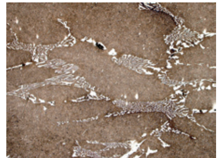
Figure 7: Microstructure of new high German die steel Martensite + Carbide, \times 100
