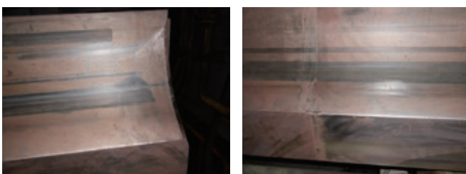
Figure 11: Surface wear condition of new crimping dies
