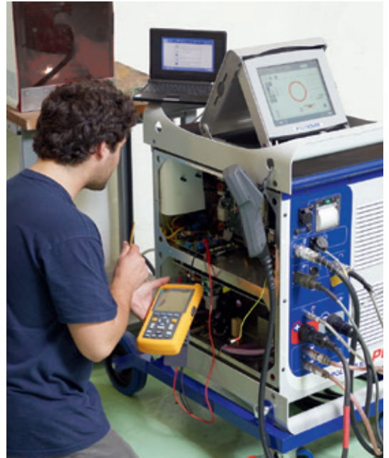
Measuring and checking a printed circuit board during a maintenance operation on a Polysoude power source
