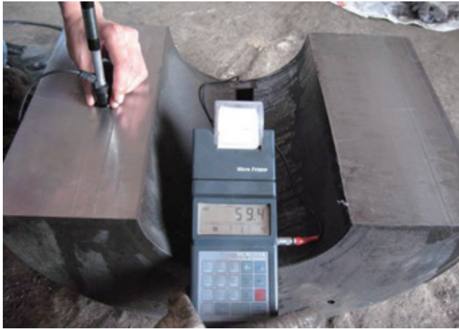
Figure 4: Field hardness testing picture of experimental cylindrical sample profile
