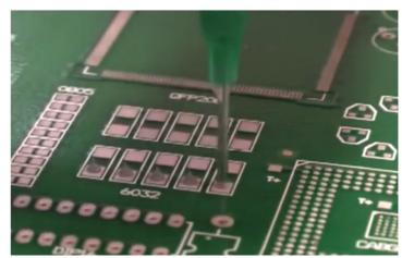
Even complex program patterns can be developed quickly using the simple point to point teach pendant. Dispense adhesive direct from syringes or optional metering valves and pressure pots. With fast indexing speeds, high accuracy and simple programming; robots are an ideal solution for most dispensing applications in a 500mm x 500mm work area. CE approved. Advanced features include work pattern array copy, end of cycle brush or wipe mode and slope dispensing.
