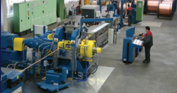
▲ A typical BWE Conform 550i installation for copper bus bar and sections
