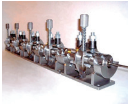
▲ Wire cleaning by BHW system
