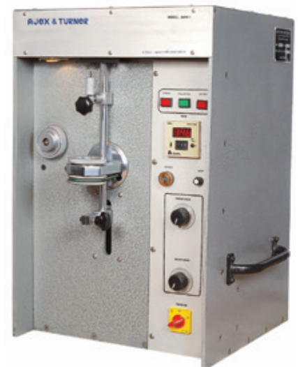
▲ In-house diamond die polishing machine
