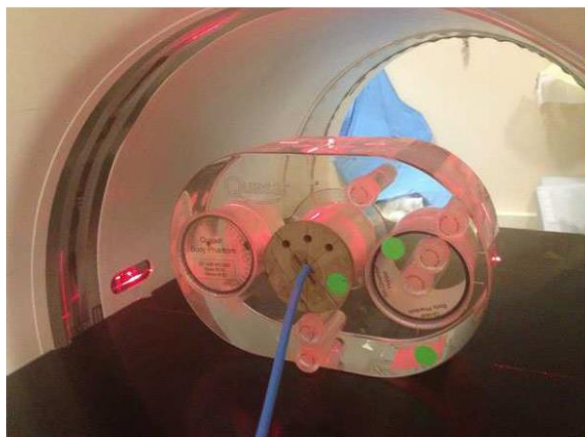
FIG. 2. QUASAR phantom used to check the accuracy of dose calculation algorithms in lung equivalent material for clinically used VMAT plans.
