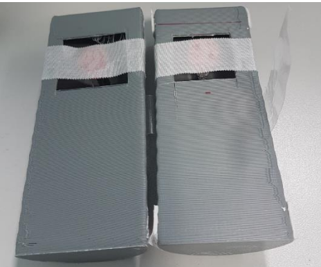
Phantom 2 3D print using ABS of hollow half cylinders to represent air to which a wax tumour of similar size was attached
