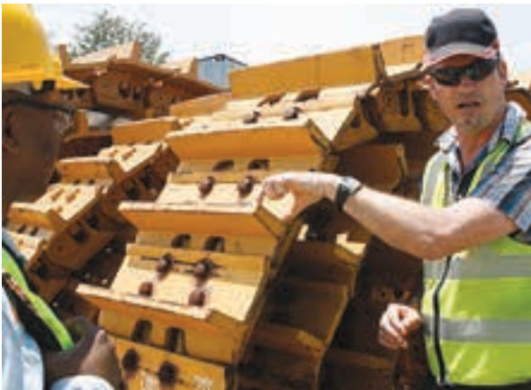
Currently the robot refurbishes track shoes for D9 (seen here), D10 and D11 Caterpillar bulldozers.
