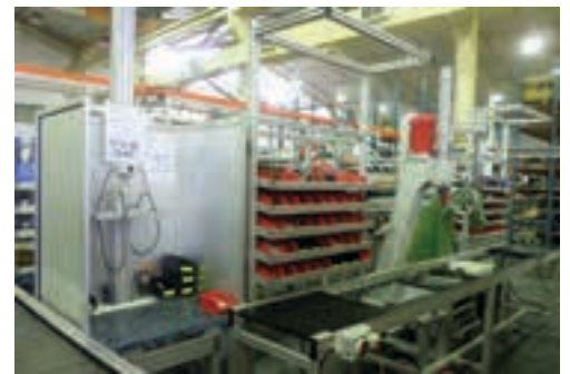
SEW-EURODRIVE Cape Town has invested in new assembly cells for geared motors to speed up production.
