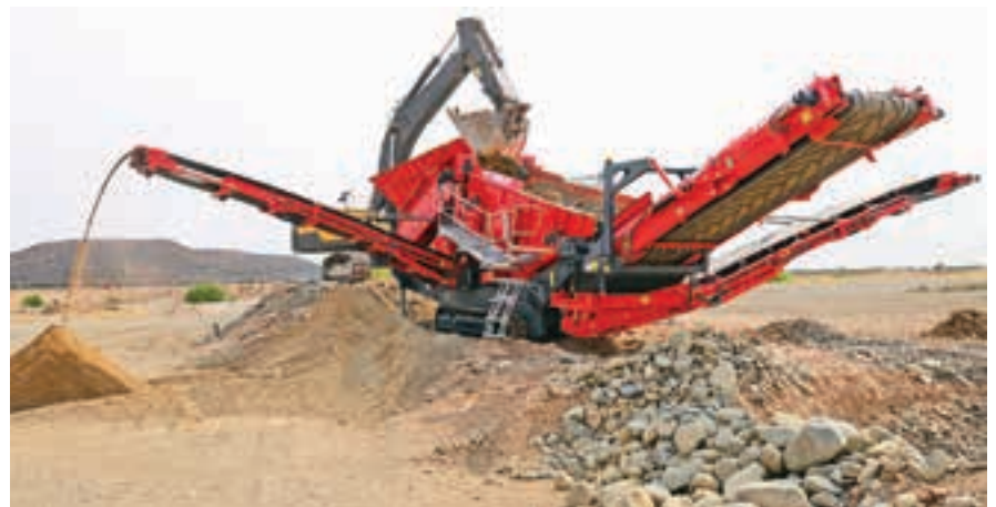
Fourie Diamante's Finlay 883+ heavy duty screen is fitted with optional hopper extensions to provide a massive 10 m 3 capacity and enable a sustained throughput of 500 t/h.
